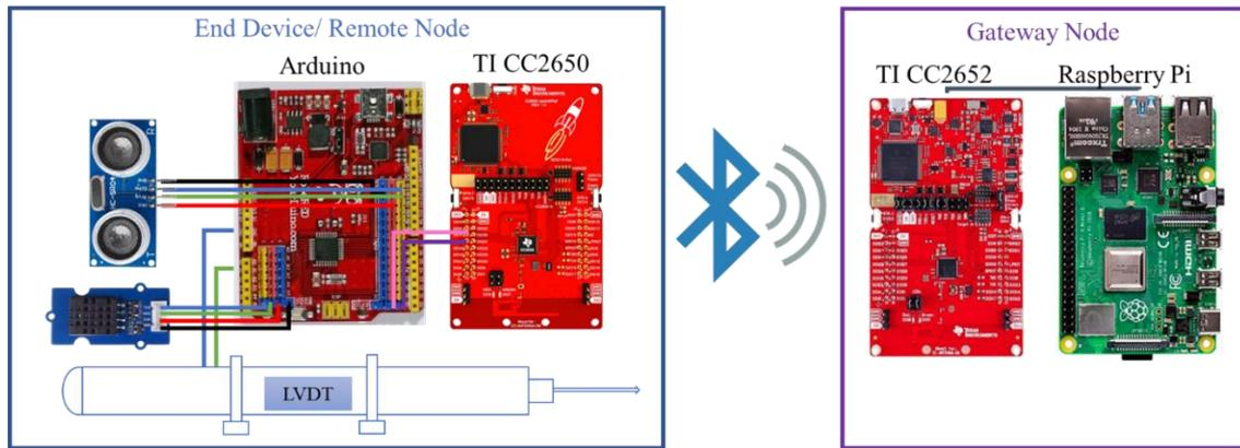
Fig. 2 Connection schematics of an end device (left) and the gateway (right)
