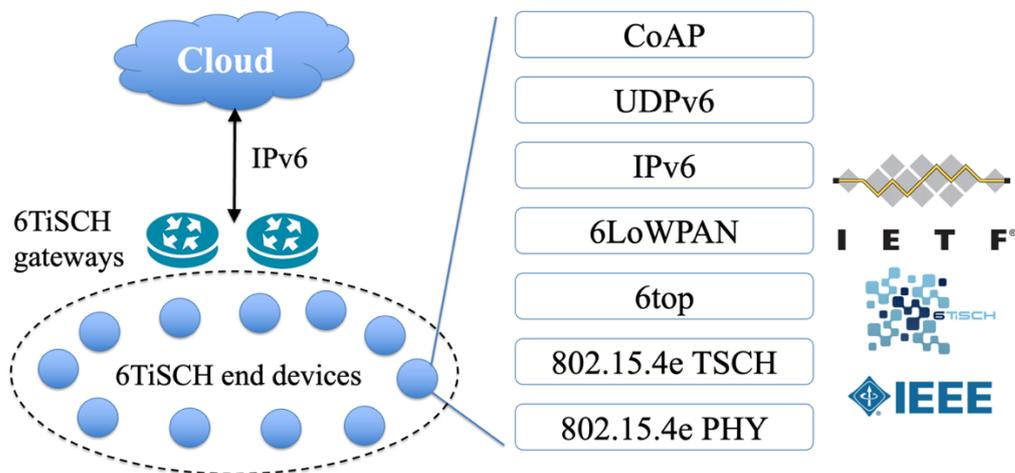
Fig. 1 Overview of the 6TiSCH network architecture (Wang *et al.* 2021)
