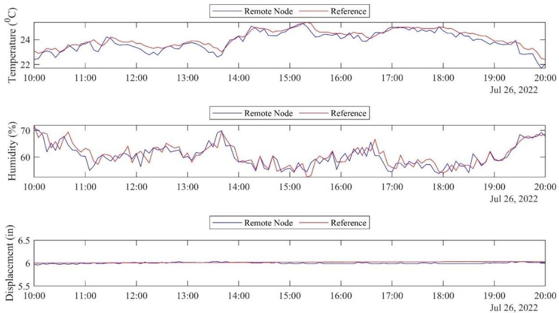
Fig. 10 Collected Data from Wireless Sensors (Remote Node) and the Reference Sensors, top: Temperature, middle: humidity, bottom: displacement
