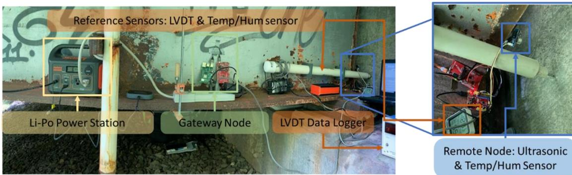
Fig. 9 Test setup of displacement monitoring campaign
