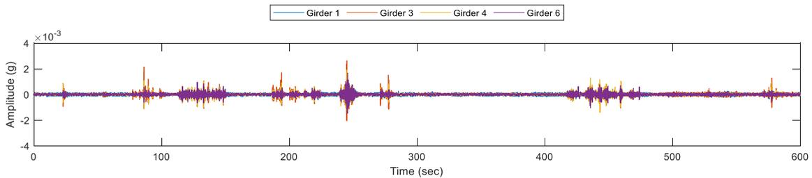
Fig. 8 Time history of vertical acceleration at S1 to S4
