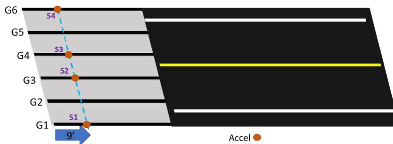
Fig. 7 Vibration testing sensor layout on the bridge
