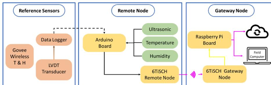
Fig. 6 Sensor schematic containing reference sensor, remote node, and gateway node
