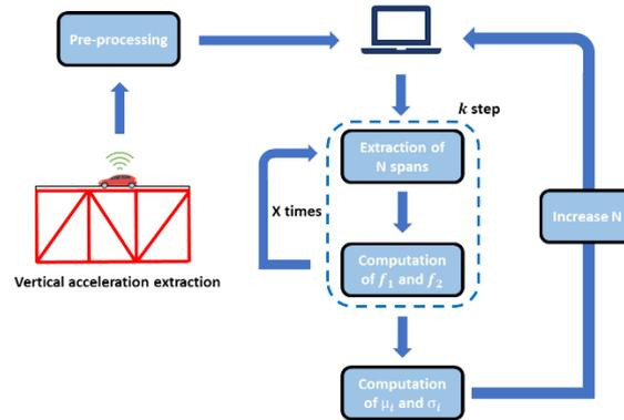
Fig. 10 Schematic description of the algorithm used for the study of the relationship between identification accuracy and number of trips taken into account while running the analysis
