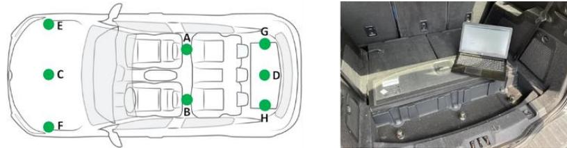
Fig. 3 On the left: schematic representation of the sensor network deployed on the diagnostic vehicle. The letters refer to the list above; on the right: placement of the three sensors inside the car trunk
