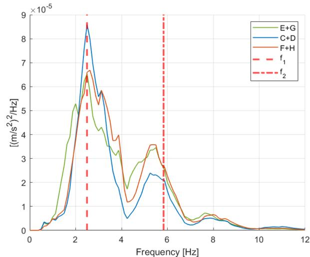
Fig. 7 PSD functions computed from three different signals, obtained summing the raw data from sensors E and G, C and D, and F and H respectively. This artifice allows to compensate the pitch motion of the car, highlighting the bridge dynamics. The red dashed lines highlight the first two bending frequencies of the bridge. Refer to Fig. 3 for the positioning of the sensors
