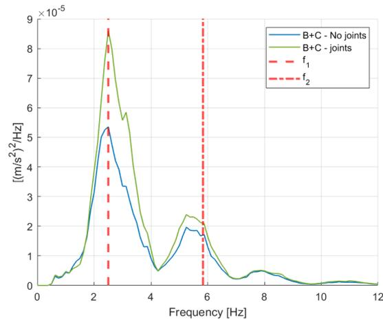
Fig. 9 Comparison of the PSD functions computed from two different signals: the green line refers to a signal obtained summing the raw data from sensors C and D; the blue line refers to a signal obtained summing the data from sensors C and D after removing the acceleration spikes in correspondence of the expansion joints (i.e., dataset B)
