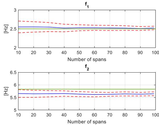
Fig. 11 Representation of mean value – blue line – and standard deviation – red dashed line – with respect to the number of crossed spans taken into account. The green line represents the target frequency. Above: 1<sup>st</sup> bending frequency; below: 2<sup>nd</sup> bending frequency
