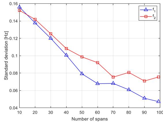
Fig. 12 Comparison of the standard deviation trends for the indirect estimation of the two natural frequencies of the bridge. On the abscissa, the number of crossed spans included in the analysis randomly extracted from data set B
