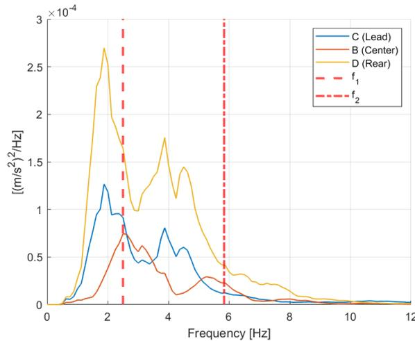
Fig. 6 PSD functions computed from sensors B, C, and D. The dashed lines highlight the first two bending frequencies of the bridge. Refer to Fig. 3 for the positioning of the sensors
