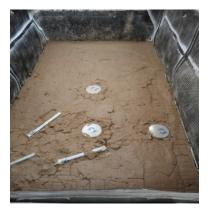
Fig. 7 Earth pressure cells
