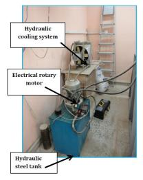
Fig. 3 Hydraulic loading system
