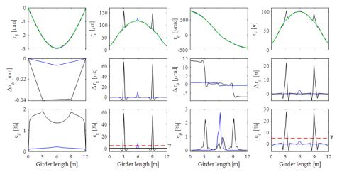
Fig. 6 From left to right: deflection, strain, inclination angle and curvature along the length of the girder. From top to bottom: girder response (r), change in girder response  $(\Delta r)$  and damage sensitive feature (e). Green dashed lines are response at no damage (only for response plots); blue and black lines are  $S_1D_2$  and  $S_2D_5$ , respectively
