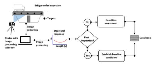
Fig. 1 Vision-based condition assessment of bridges
