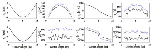
Fig. 9 Girder response (r) from raw (blue line) and pre-processed (black line)  $r_{max}$  values at  $N_1F_1$  (top) and  $N_3F_1$  (bottom) combinations. From left to right: deflection  $(r_\delta)$ , strain  $(r_\epsilon)$ , inclination angle  $(r_\theta)$  and curvature  $(r_\epsilon)$
