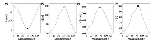
Fig. 5 Response histories of (a) deflection; (b) strain; and (d) curvature at the mid-span of the girder; and (c) inclination angle next to the left support derived from nodal displacements. 'x' marks the maximum absolute response value
