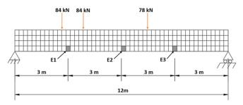
Fig. 4 A sketch of the numerical model and load locations at 50th measurement step
