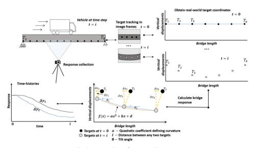
Fig. 2 Generation of structural response
