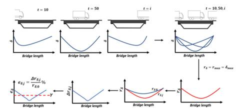
Fig. 3 Damage detection technique from vertical deflections
