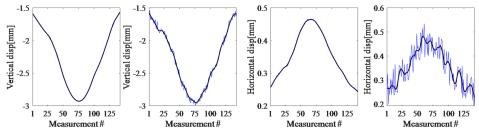
Fig. 7 Raw (blue line) and pre-processed (black line) displacements of a target at the midspan of the girder. Left to right: Vertical displacements at  $N_1F_1$ ,  $N_3F_1$ , and horizontal displacements at  $N_1F_1$ ,  $N_3F_1$
