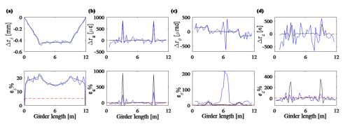
Fig. 10  $\Delta r$  and e for deflection, inclination, strain and curvature (from left to right) at damage scenarios  $S_3D_5$  at  $N_1F_1$  (black lines) and  $N_3F_1$  (blue lines) combinations. Red dashed line is the damage threshold
