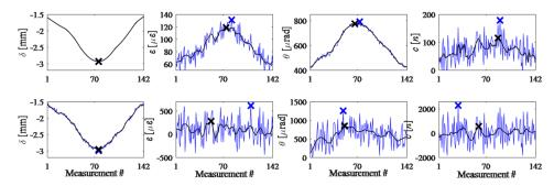
Fig. 8 From left to right: Measurement histories of raw (blue line) and pre-processed (black line) deflections, strains and curvatures at the mid-span of the girder, and inclination angles next to the left support derived from pre-processed target displacements at  $N_1F_1$  (top) and  $N_3F_1$  (bottom) combinations. 'x' indicates the absolute maximum response value
