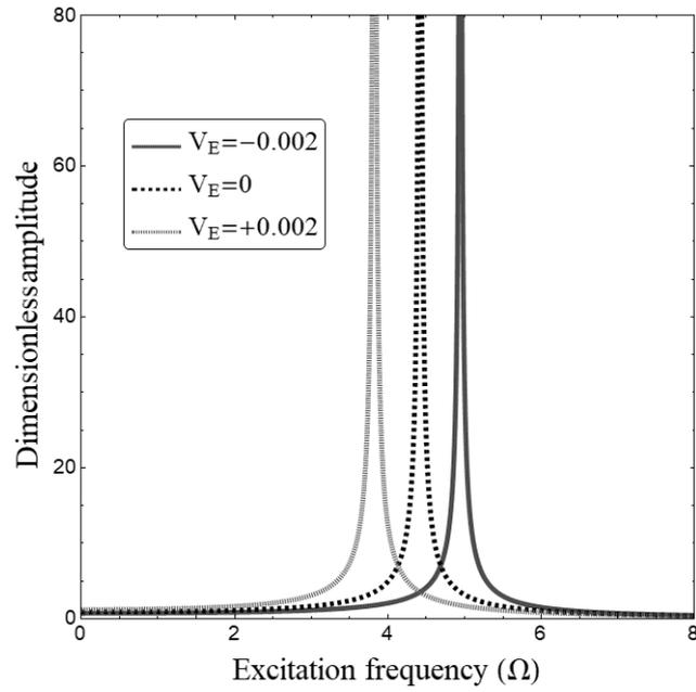
Fig. 4 Effect of applied electric voltage on response curves ( $a/h=20$ ,  $\mu=0.2$ ,  $\lambda=0$ ,  $e_0=0.2$ )
