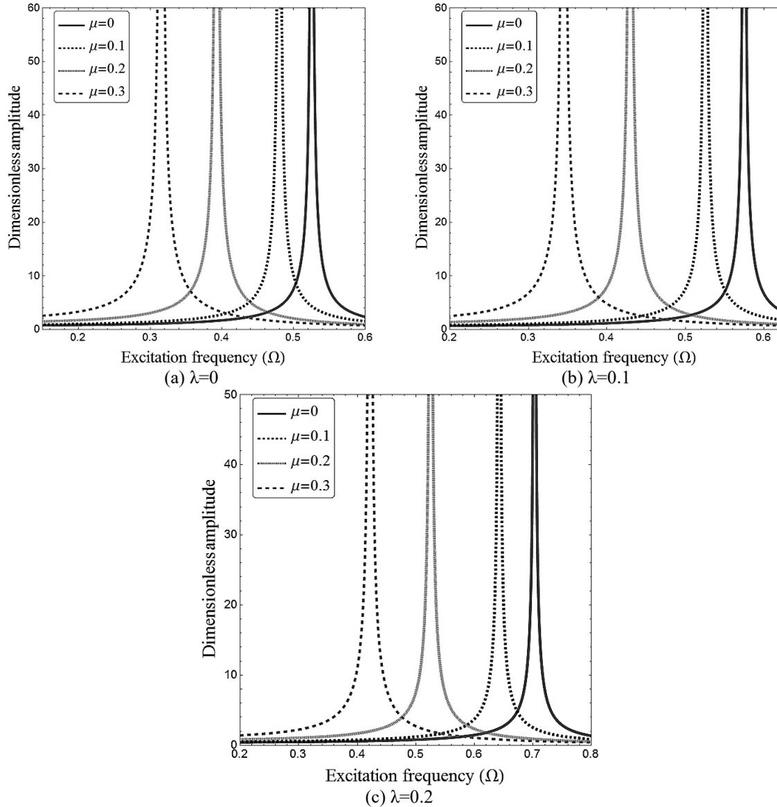
Fig. 3 Effect of nonlocal and strain gradient factors on response curves of nano-size plate ( $a/h=10$ ,  $K_w=0$ ,  $K_p=0$ ,  $e_0=0.5$ )
