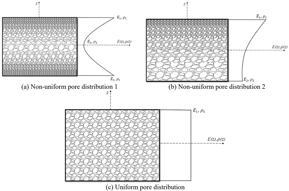
Fig. 1 Pore types along the thickness direction
