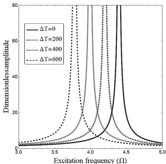
Fig. 8 Response curves of the nano-size plate according to a variety of temperature changes ( $a/h=20$ ,  $\mu=0.2$ ,  $e_0=0.2$ )
