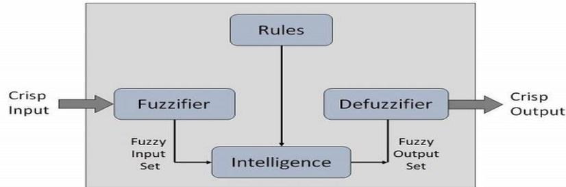
Fig. 1 The system architecture of the fuzzy-rule-based decision system
