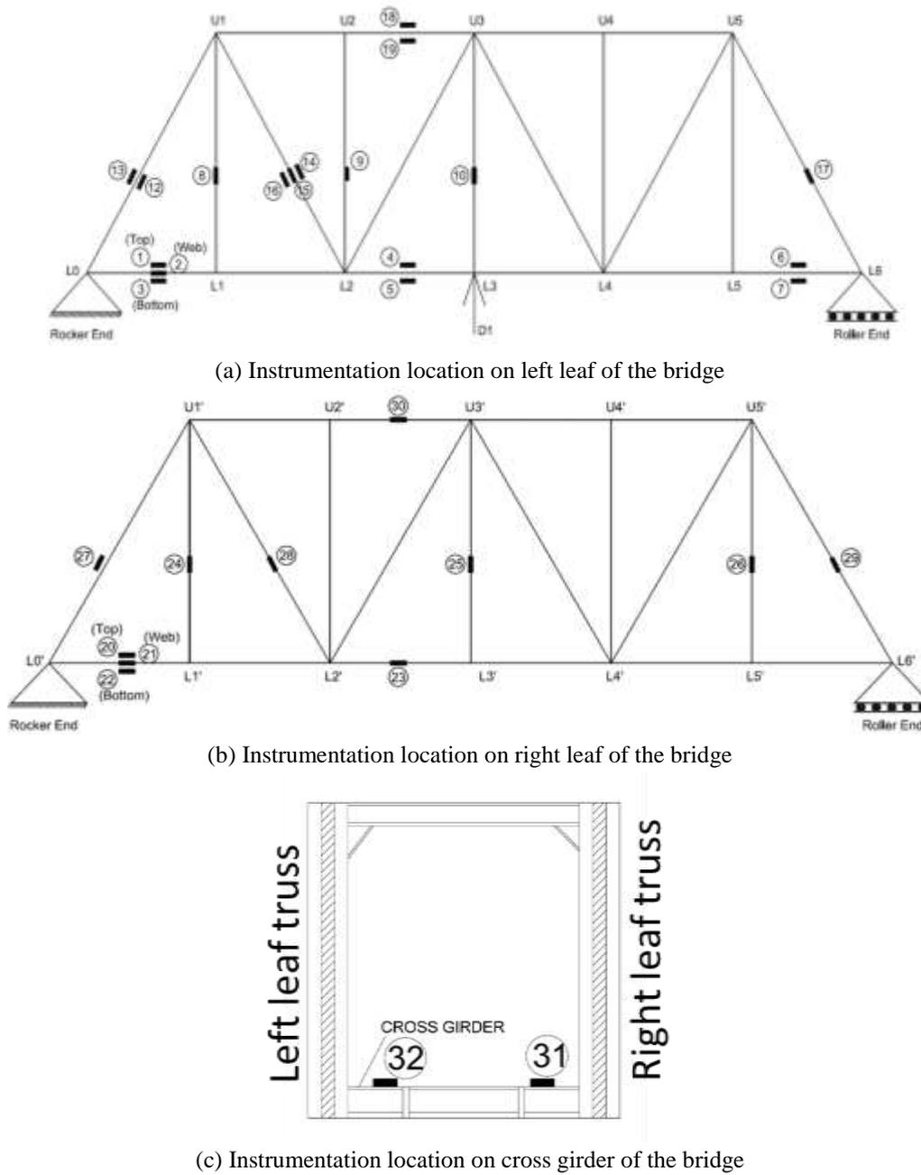
Fig. 3 Schematic representation of Instrumentation locations in the bridge
