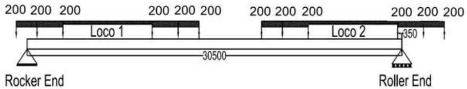
All loads in kN and All dimensions are in mm
