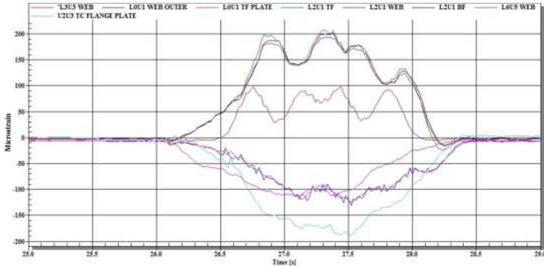
Fig. 16 Variation of strain for Uniform speed case
