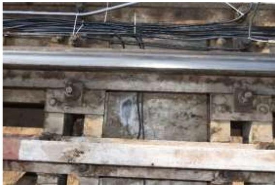
Fig. 6 Strain gage instrumented in cross girder
