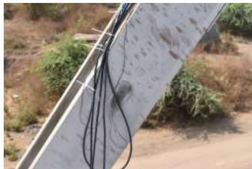
Fig. 4 Strain gage instrumented in diagonal member
