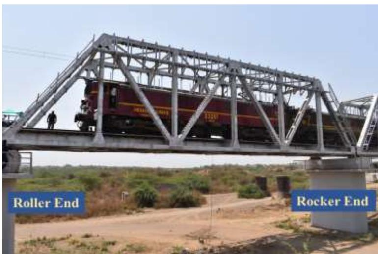
Fig. 14 Dual loco placed for maximum shear case
