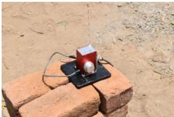
Fig. 7 Instrumentation of displacement transducer at midspan
