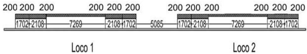
All loads in kN and All dimensions are in mm
