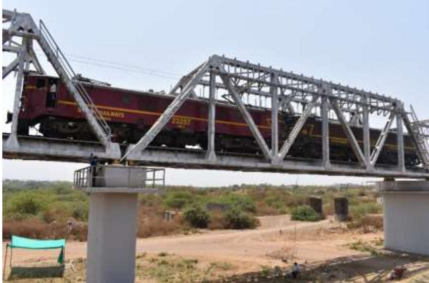
Fig. 9 Coupled loco (WAG 5) used for the experimental investigations
