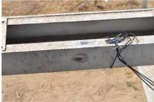
Fig. 5 Strain gage instrumented in bottom chord
