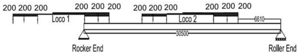
All loads in kN and All dimensions are in mm
