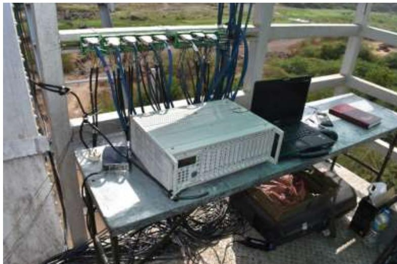
Fig. 8 High speed data acquisition system for measuring the responses
