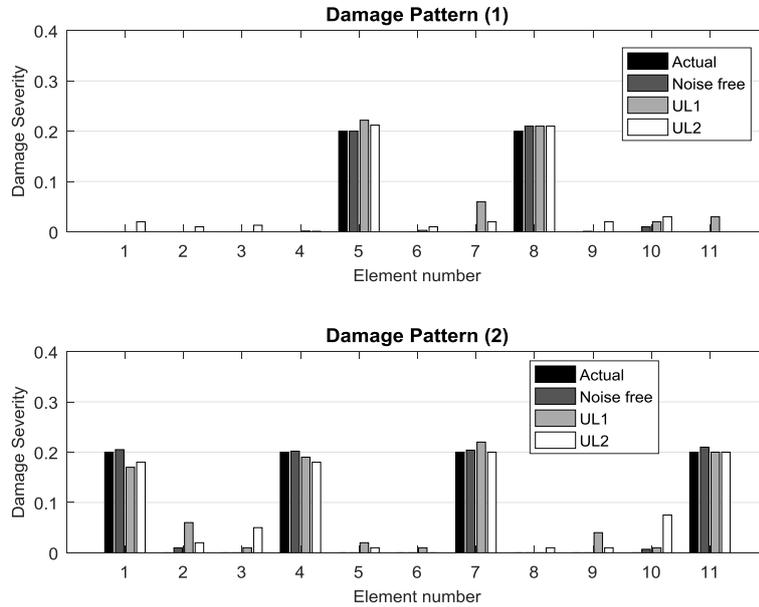
Fig. 4 Results of second stage for the three-story plane steel frame with two uncertainty level
