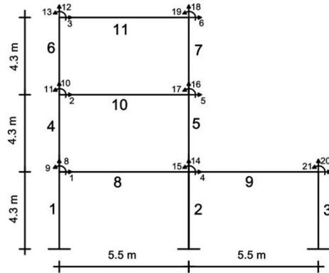
Fig. 3 Three-story plane frame with the finite element model
