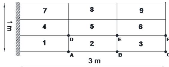
Fig. 5 The cantilever plate with finite element model
