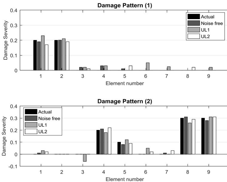
Fig. 6 Results of second stage for the cantilever plate with two uncertainty level
