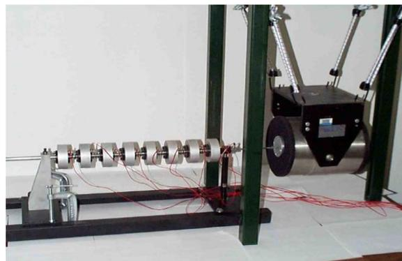
Fig. 7 Experimental 8 DOFs system with excitation shaker attached (Duffey *et al.* 2001)
