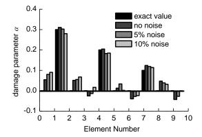
Fig. 7 Multi-damage identification results under different noise levels
