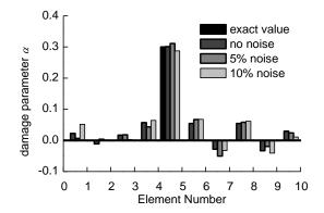
Fig. 4 Single damage identification results under different noise levels
