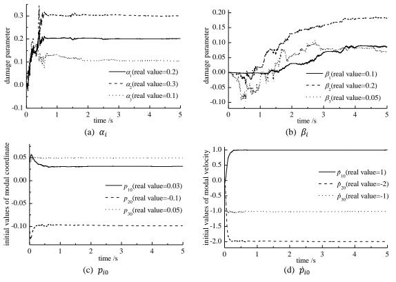
Fig. 1 Convergence curve of state variables (noise level is 15%)
