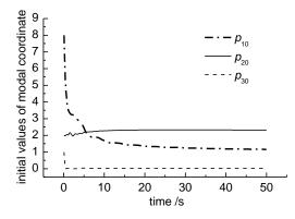
Fig. 5 Convergence curve of the initial values of modal coordinates in the state vector of EKF
