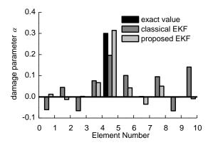
Fig. 6 The influence of Tikhonov regularization to damage identification results
