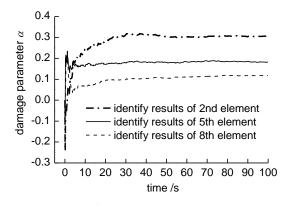
Fig. 8 Convergence curve of the damage parameters under 5% noise level
