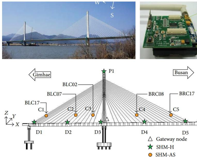
Fig. 2 Wireless Sensor deployment in the Hwamyung Bridge (Ho *et al.* 2012)
