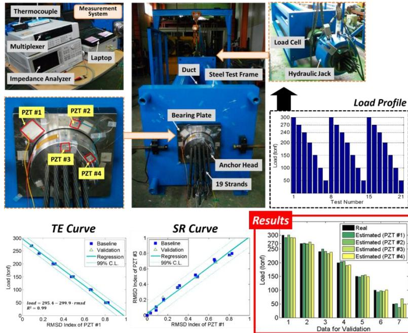
Fig. 6 Tensile force estimation and nearby damage detection with multiple piezoelectric sensors on 19-strand anchorage system (Min *et al.* 2016)
