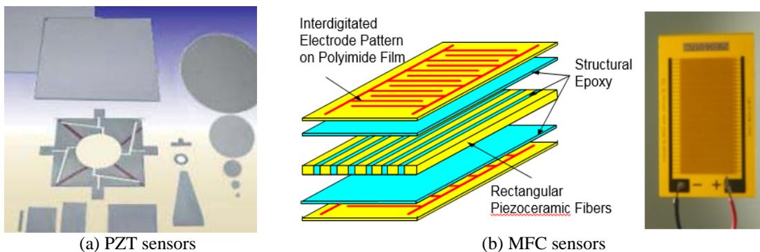
Fig. 1 Various piezoelectric sensors
