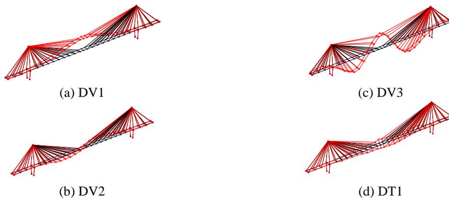
Fig. 14 Example mode shapes and MAC values correlating to FE model analysis (Spencer *et al.* 2016)
