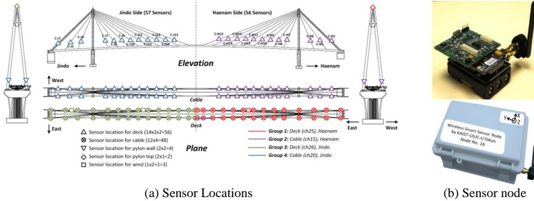
Fig. 13 Sensor nodes deployed on the second Jindo Bridge (Spencer *et al.* 2016)
