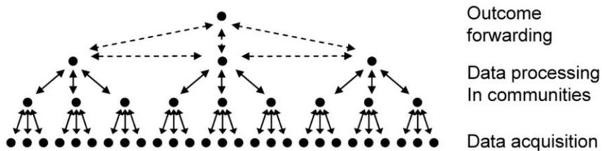
Fig. 7 Decentralized processing scheme (Nagayama *et al.* 2010)
