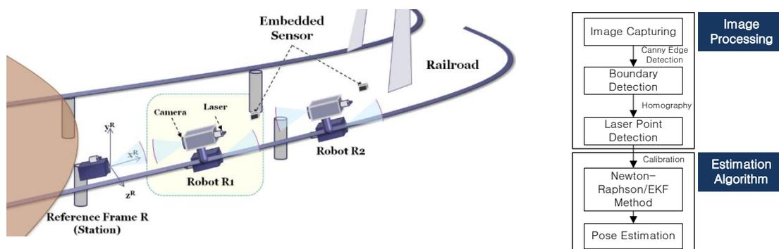
Fig. 4 Schematic diagram of vision-based displacement measurement system (Myung *et al.* 2011)
