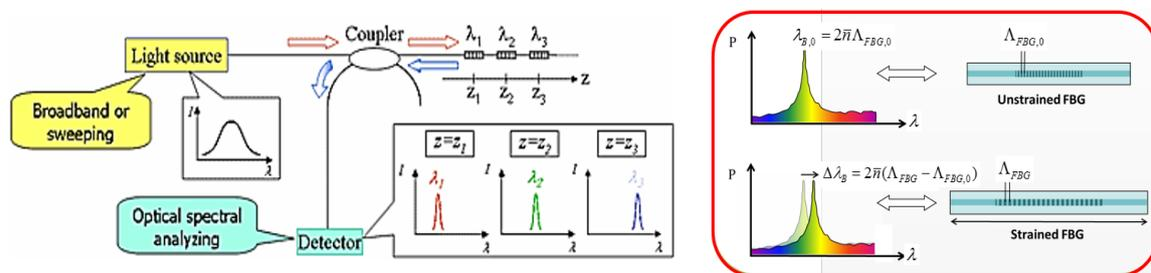
Fig. 3 Schematic of FBG sensor system
