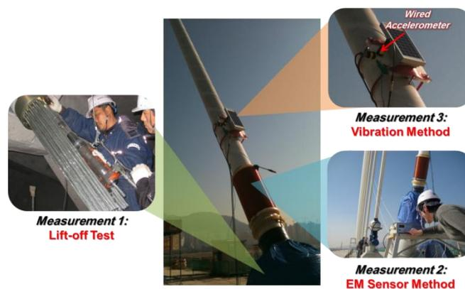
Fig. 16 Test setup for comparative study
