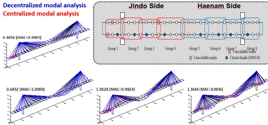
Fig. 8 Decentralized identification of modal properties in Jindo bridge
