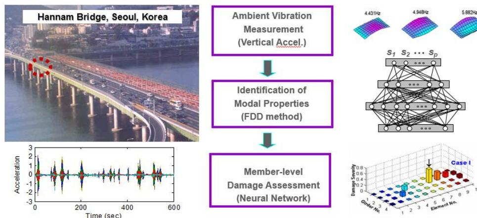
Fig. 5 Vibration-based damage detection on Hannam Grand Bridge
