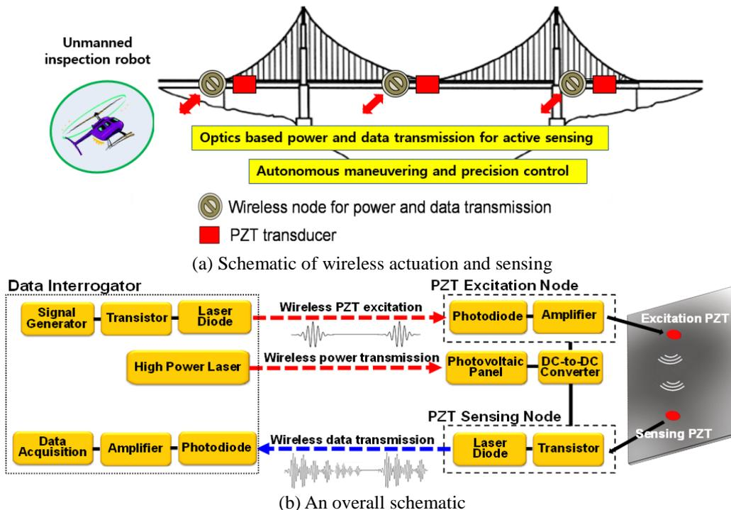
Fig. 9 Optics-based wireless guided wave generation and non-contact sensing (Park *et al.* 2010)
