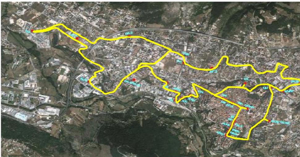
Fig. 1 Map of L'Aquila with evidence, in yellow line, of the experimental optical network connecting the different SHM systems for strategic and monumental buildings
