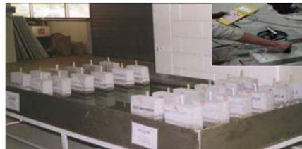
Fig. 2 Test setup of Corrosion Rate Test (Lollipop Test)
