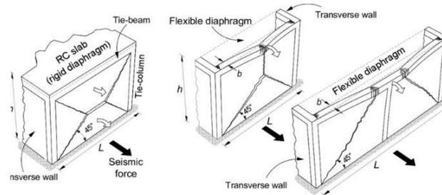
Fig. 6 The out-of-Plane failure mechanism of masonry wall (Source: <http://achyutpauwel.com.np/>)
