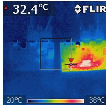
Fig. 11 Thermal performance of two SHM Endpoints. The left SHM Endpoint only has the AWM activated while the right SHM Endpoint has both the AWM and the SHM Sensor activated
