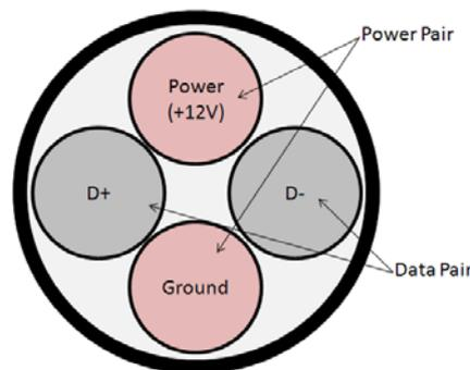
Fig. 9 BILBO Network bus cable cross-section
