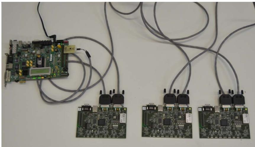
Fig. 8 Laboratory setup of a BILBO Subnetwork
