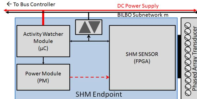
Fig. 4 Bi-operator architecture of the SHM Endpoint
