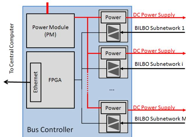
Fig. 5 Architecture of the Bus Controller
