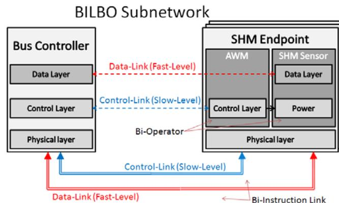
Fig. 7 Point-to-point communication protocol between the Bus Controller (left) and the SHM Endpoint systems (right)
