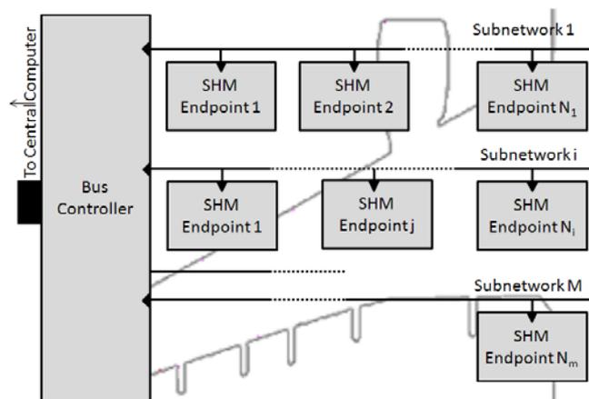
Fig. 3 Representation of a BILBO Network composed of a Bus Controller and many BILBO Subnetworks, which contain multiple SHM Endpoints
