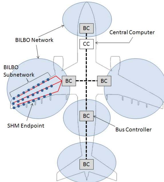
Fig. 2 Representation of a BILBO Network installation on-board an aircraft. The SHM Endpoints are contained in BILBO Subnetworks, which are gathered in BILBO Networks. Bus Controllers connect the BILBO Networks with the Central Computer using the main communication system of the aircraft
