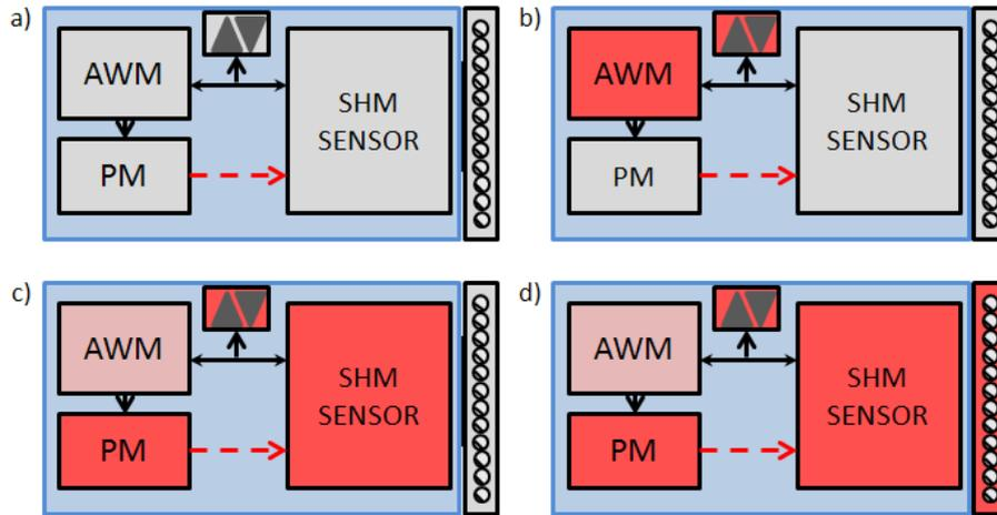
Fig. 6 Four power modes available in the SHM setup: (a) NET\_OFF\_MODE, (b) SLEEP\_MODE, (c) ACTIVE\_MODE and (d) TESTING\_MODE
