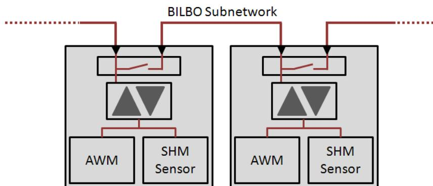
Fig. 10 SHM Endpoints power connections to the BILBO Subnetwork bus
