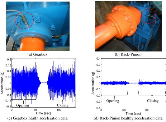
Fig. 5 Sensors on gearbox and rack-pinion with corresponding sample acceleration data
