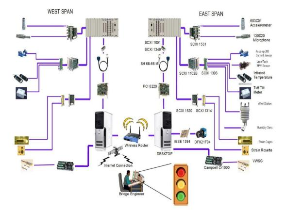
Fig. 4 Sensor network used in the movable bridge project
