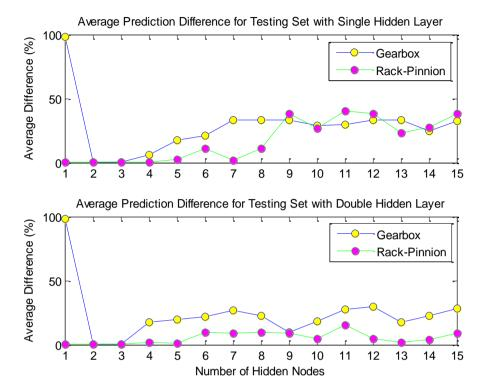
Fig. 8 Variation of Prediction Performance depending of the Network Architecture for Testing Set
