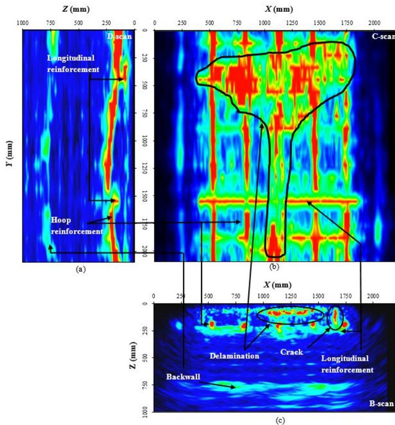
Fig. 9 UST scan sets of Area II: (a) D-scan, (b) C-scan, and (c) B-scan
