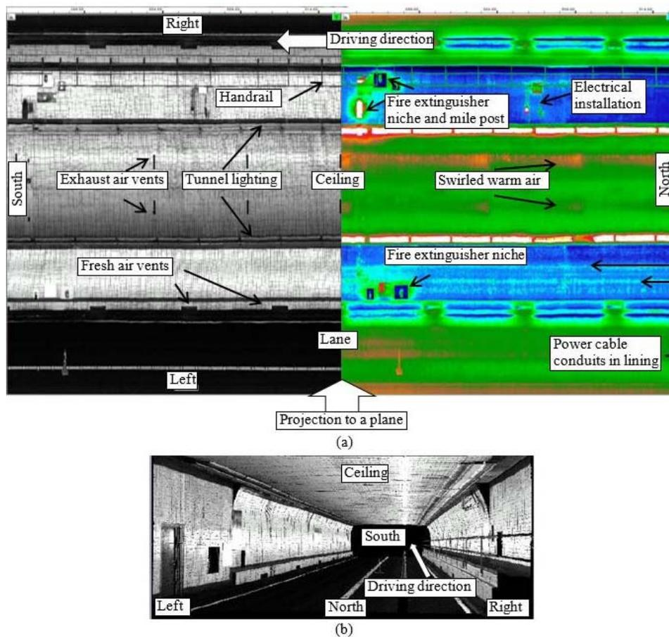
Fig. 7 (a) Typical features in SPACETEC survey data, and (b) 3D view of scan data which is calculated from survey data (not video data)
