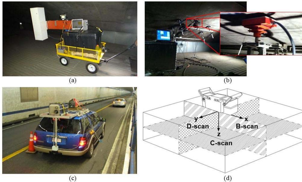
Fig. 1 NDT equipment: (a) noncontact A.C. GPR on cart, (b) G.C. GPR on BAM ZFP-scanner, (c) noncontact vehicle-mounted SPACETEC equipment, and (d) UST with inspection planes
