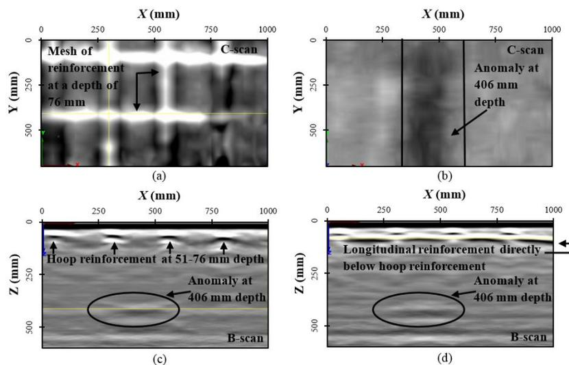
Fig. 5 GPR scan sets: (a)-(b) C-scans at two different locations, taken at 76 mm and 406 mm, respectively, and (c)-(d) B-scans at two different locations
