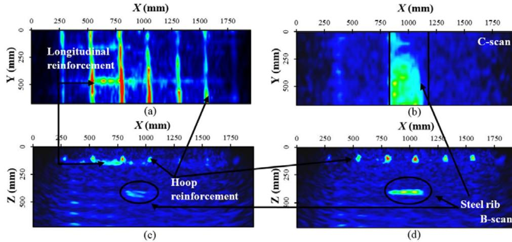
Fig. 6 UST scan sets: (a)-(b) C-scans at two different locations, taken at 105 mm and 409 mm, respectively, and (c)-(d) B-scans at two different locations
