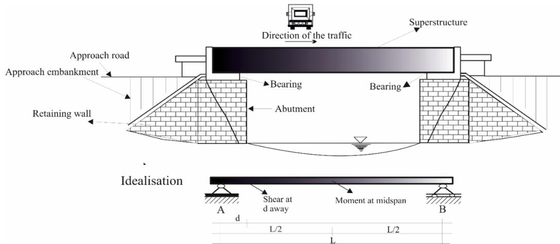
Fig. 2 Simple span bridge idealization and the locations of shear and moment
