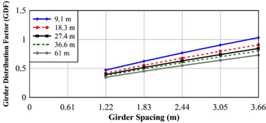
Fig. 7 Girder distribution factors of moment for two or more traffic lanes.
