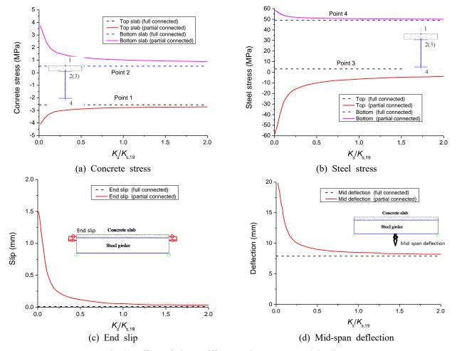
Fig. 11 Effect of shear stiffness under concentrated loading
