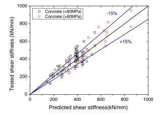
Fig. 7 Comparison between predicted and tested shear stiffness
