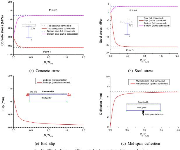
Fig. 12 Effect of shear stiffness under temperature difference loading
