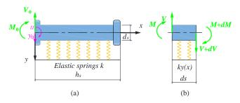
Fig. 5 Analytical model of stud in concrete: (a) stud on an elastic foundation and (b) differential element of length dx
