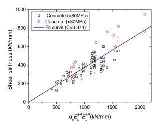
Fig. 6 Fitting of shear stiffness
