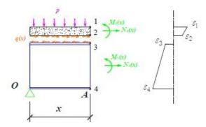
Fig. 9 Internal force and strain state for segment x under uniformly distributed load
