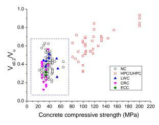
Fig. 3 The relation of  $V_{s0.2}/V_u$  and concrete strength for shear stud in various types of concrete
