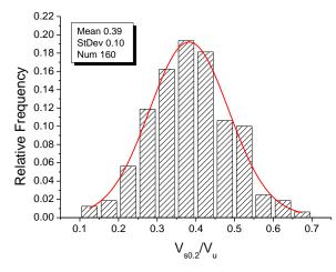
Fig. 4 The frequency distribution of  $V_{s0.2}/V_u$  for studs in concrete ( $f_c < 80$  MPa)
