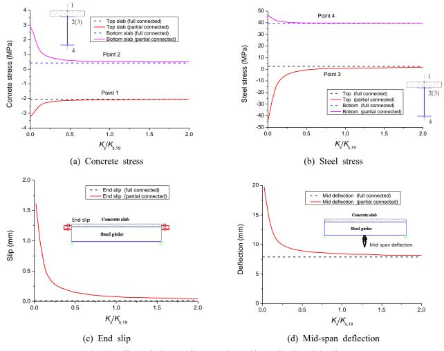
Fig. 10 Effect of shear stiffness under uniform distributed loading
