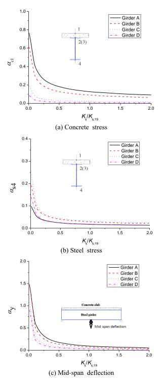
Fig. 13 Effect of shear stiffness for different composite girders
