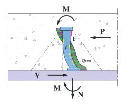
Fig. 1 Shear transfer mechanism in push-out test
