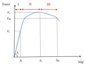
Fig. 2 Typical load-slip curve for studs in push-out test
