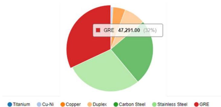
Fig. 3 Rate of used materials except pipe
