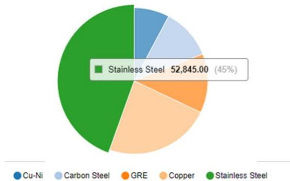
Fig. 5 Rate of materials of pipe at living quarter
