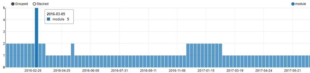
Fig. 20 Number of modules that start steel cutting per schedule
