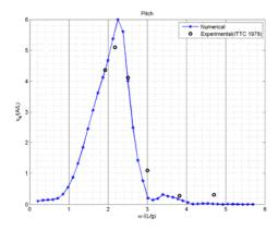
Fig. 3 Comparison of pitch response of S175 container ship at  $F_n$ =0.275 and  $\beta$ =180 deg
