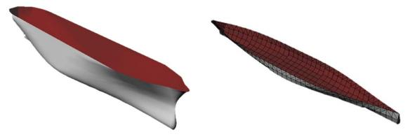
Fig. 1 Hull form (Left) and panel mesh(right) of S175ContainerShip
