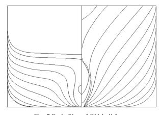
Fig. 7 Body Plan of C11 hull form
