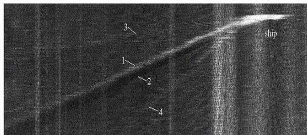
Fig. 1 Ship wakes of SAR image
