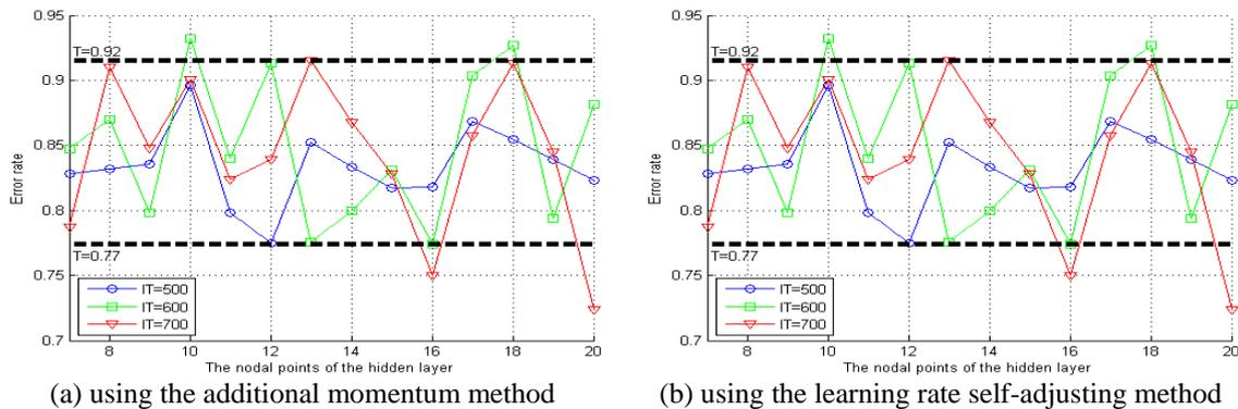
Fig. 8 the relationship between the classification error and the nodal points of the hidden layer
