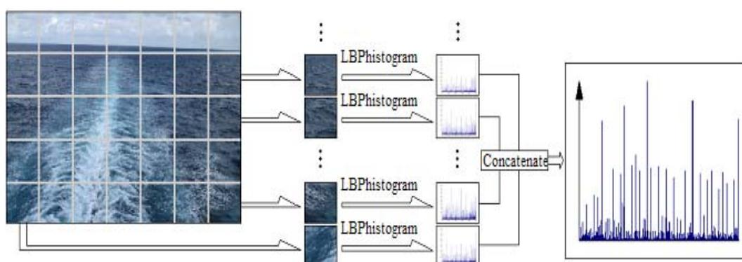
Fig. 5 Ship wake description with sub-area LBP histograms features
