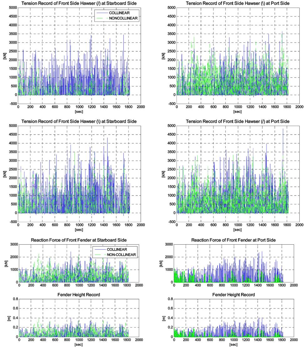
Fig.7 Time histories of side hawser tensions and fender reaction forces & fender heights
