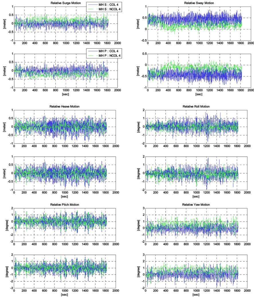
Fig. 4 Relative response time histories for 6 DOF motions (MHP = mobile harbor port side with respect to the container ship, MHS = mobile harbor star-board side) The blue (solid) line is for collinear case and the green (dash-dot) line is for non-collinear case (new)
