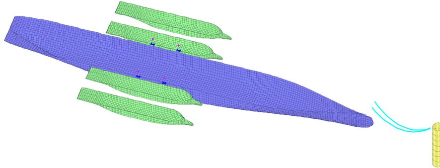
Fig. 2 Schematic view of the mobile harbor system and panels for hydrodynamic calculations
