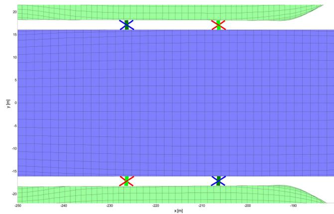
Fig. 6 Enlarged X-Y plan view of 4 sets of cross hawsers and fenders
