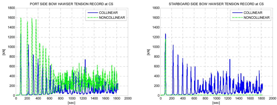
Fig. 5 Tension records for both bow hawsers
