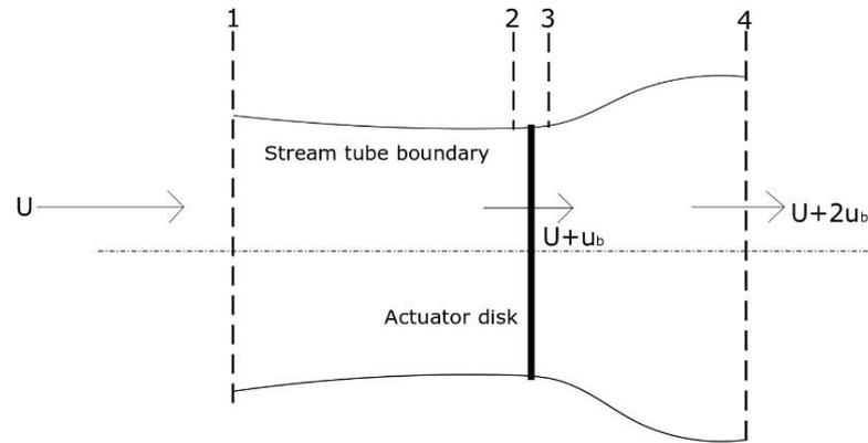
Fig. 4 A visual representation of the Actuator Disk Model
