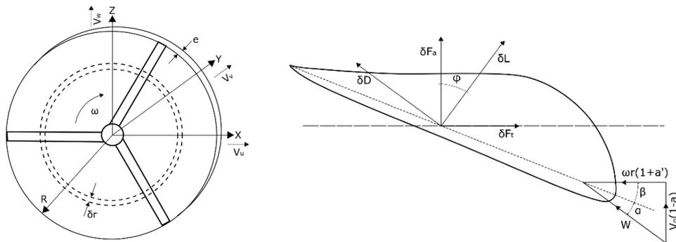
Fig. 5 (a) Disc Model with Blade Element and Regions and (b) Blade Element Velocities and Forces
