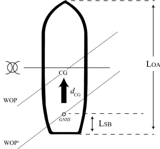
Fig. 7  $d_{CG}$  is the distance between the ship's bridge ( $L_{SB}$ ) and the ship's longitudinal Centre of gravity ( $L_{CG}$ )
