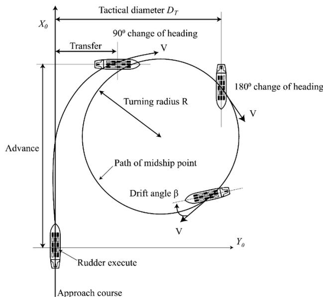
Fig. 3 Typical manoeuvring characteristic of a ship (ITTC 2002)
