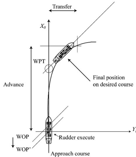
Fig. 5 This study's concept (ship's heading and course are the same at the end of alteration)
