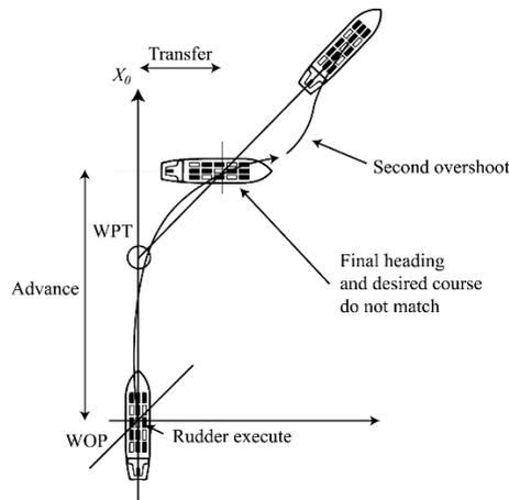
Fig. 2 Advance transfer technique principle (Anwar 2015)
