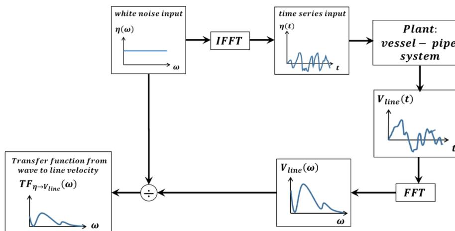
Fig. 5 System identification methodology
