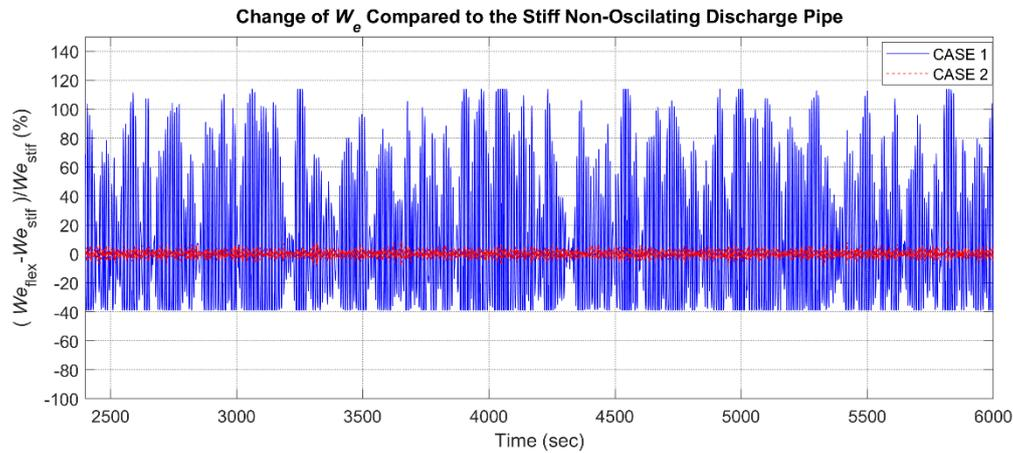
Fig. 16 Change of the discharged CO<sub>2</sub> Weber numbers for two different sea states
