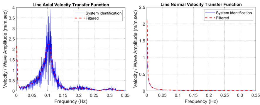
Fig. 11 Line’s axial and normal Velocity Transfer Function (VTF) from system identification
