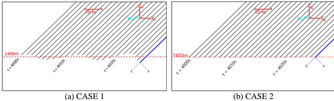
Fig. 12 Discharge pipe's position evolutions for two different sea states
