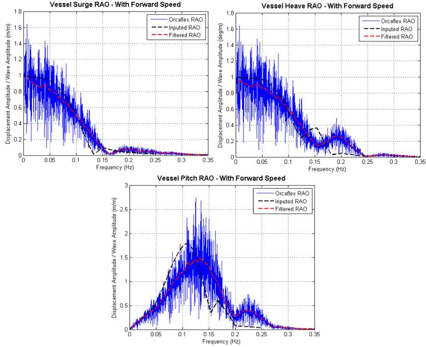
Fig. 10 System identification result of vessel’s RAO with forward speed
