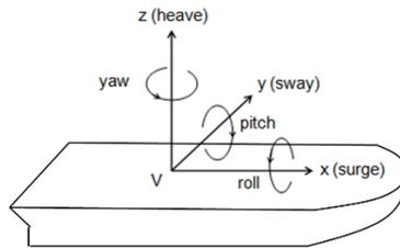
Fig. 2 Definition of the vessel's degrees of freedom
