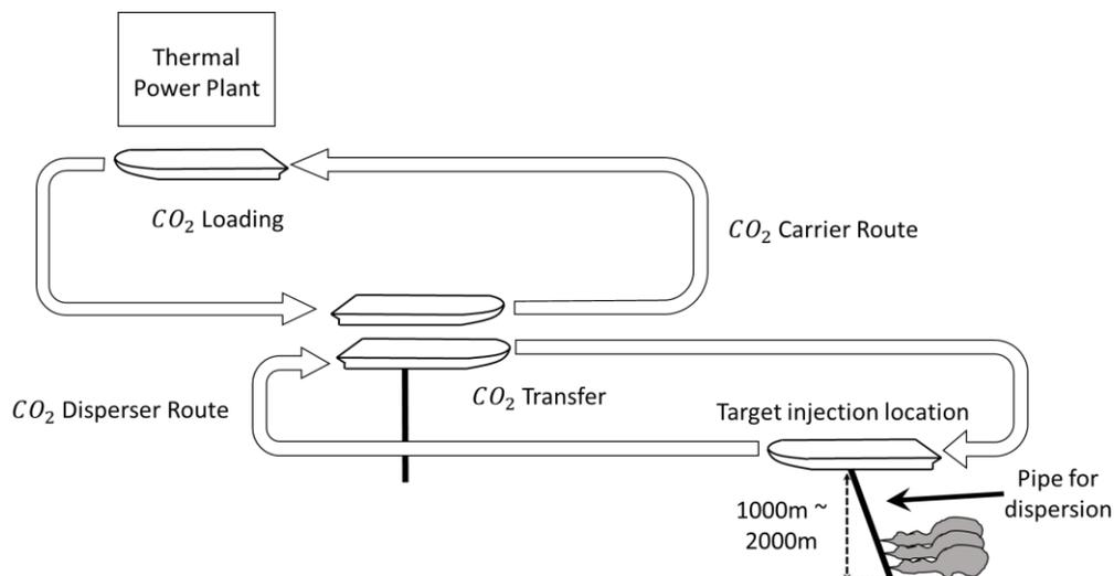
Fig. 1 Dissolution type injection method (Ozaki *et al.* 1997)
