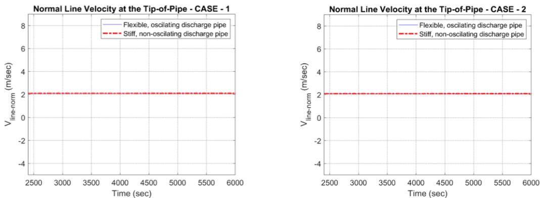
Fig. 14 Normal line velocity time history at the tip-of pipe for two different sea states
