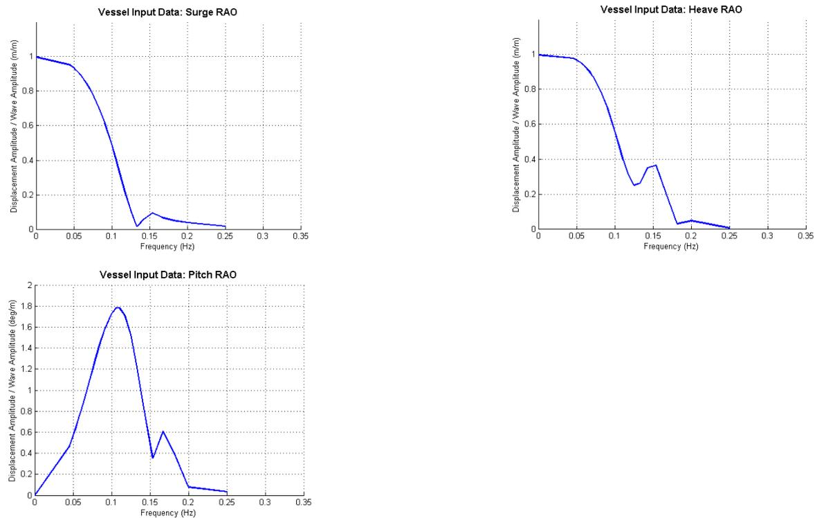
Fig. 7 Vessel's input surge, heave, pitch RAOs
