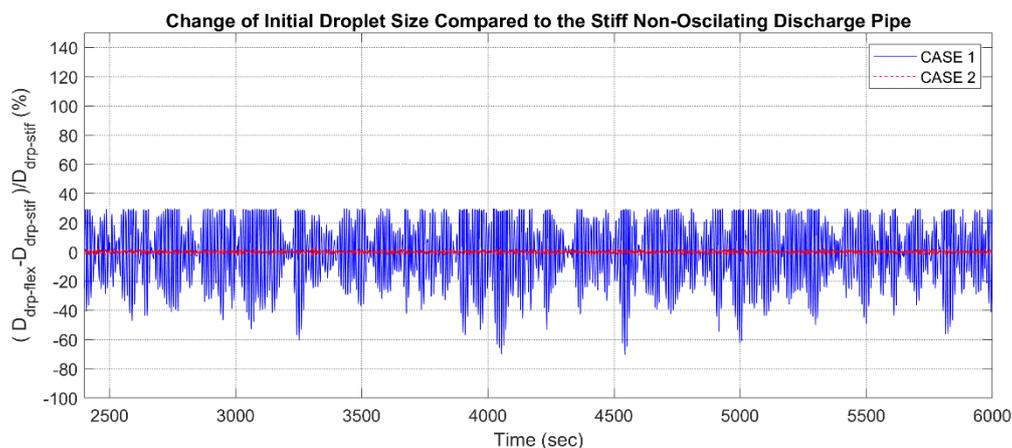
Fig. 15 Change of the discharged CO<sub>2</sub> droplet sizes for two different sea states
