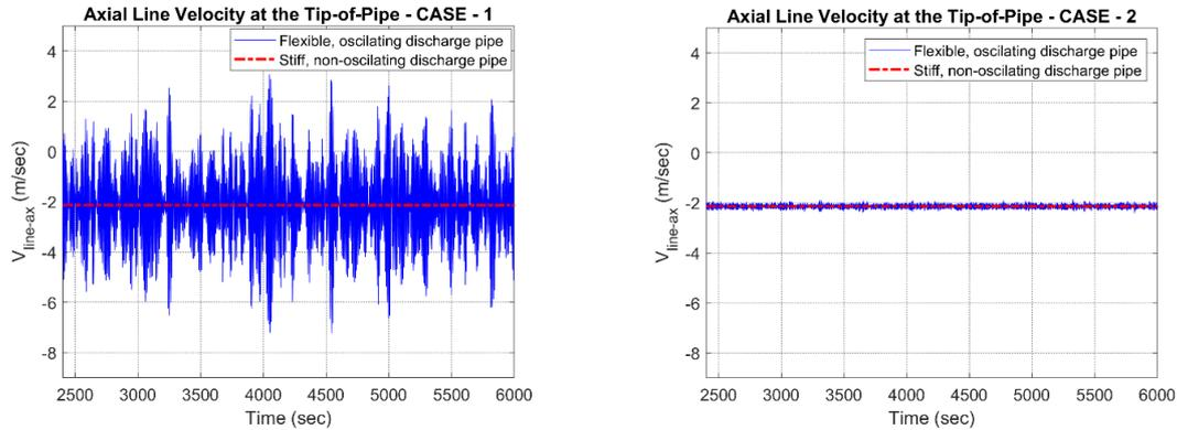
Fig. 13 Axial line velocity time history at the tip-of pipe for two different sea states
