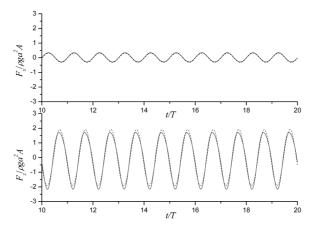
Fig. 16 Histories of hydrodynamic force on cylinder 1 at  $k_0a = 1.0$  ..... linear; —— linear plus second order
