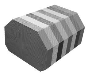
Fig. 4 Numerical grid for three-dimensional simulations
