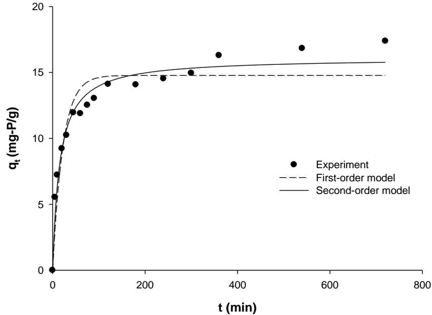
Fig. 2 Plot of kinetic adsorption of phosphate onto TiO<sub>2</sub> adsorbent
