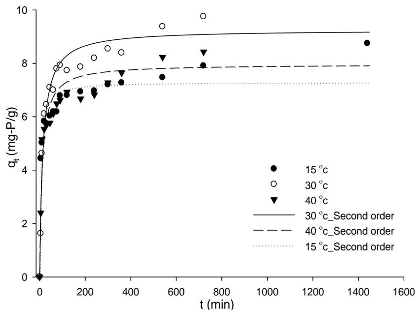
Fig. 4 The influence of temperature on phosphate adsorption onto  $\text{TiO}_2$  adsorbent
