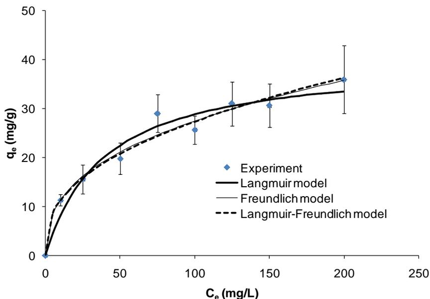
Fig. 1 Phosphate adsorption onto mesoporous TiO<sub>2</sub>
