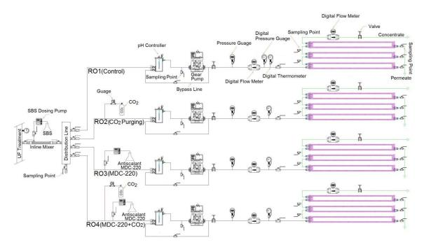
Fig. 1 Schematic diagram of the RO modules
