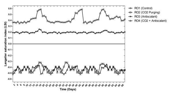
Fig. 3 Comparison between LSI data of all RO modules
