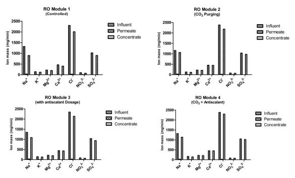
Fig. 4 Ion mass balance of RO modules
