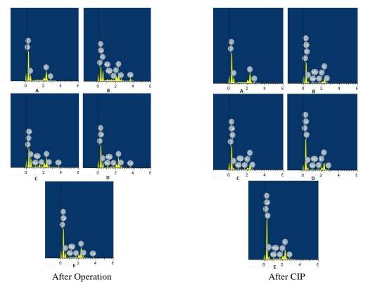
Fig. 7 EDS spectra of virgin (A), control (B),  $CO_2$  injected (C), Antiscalant dosed (D), Antiscalant dosed +  $CO_2$  injected (E) membrane
