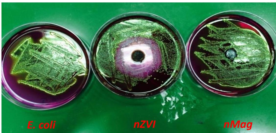
Fig. 7 (a) Control sample, (b) inhibitory zones of the nZVI pellets, (c) inhibitory zones of the nMag pellets
