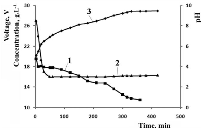
Fig. 3. Changes of voltage in the circuit, pH and concentration of  $\text{Cl}^-$  ions in the lysine solution depending on time in the process of lysine transformation from hydrochloride into basic form at  $0.6 \text{ mol.L}^{-1}$  concentration of lysine hydrochloride in the initial solution.
