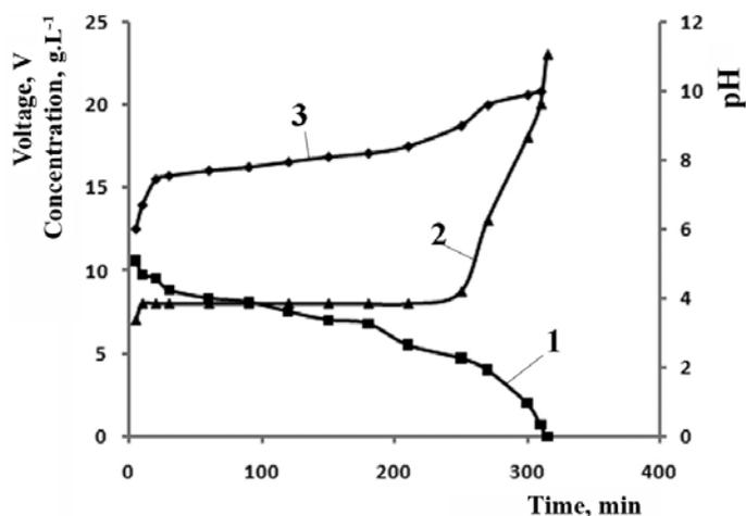
Fig. 4 Changes of voltage in the circuit, pH and concentration of  $\text{Cl}^-$  ions in the lysine solution in the process of hydrochloride (concentration  $0.3 \text{ mol.L}^{-1}$ ) transformation into zwitterionic form in a two-chamber electro dialyzer depending on time.
