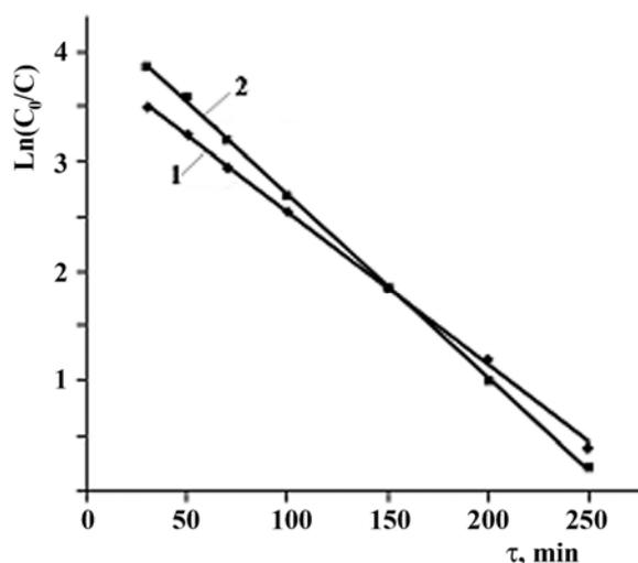
Fig. 5 Kinetic curves of lysine exchange from monohydrochloride to zwitterionic form in the process of electromembrane transformation.
