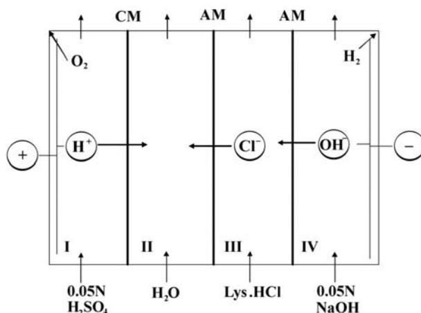
Fig. 1 Scheme of a four-chamber electro dialyzer
