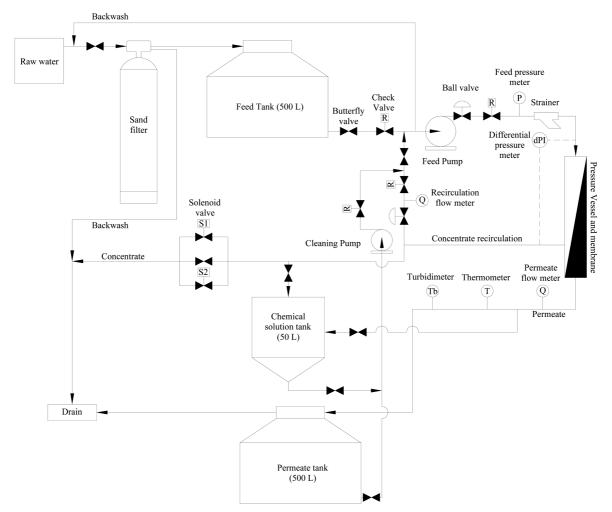
Fig. 1 Flow diagram of UF pilot plant
