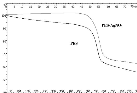
Fig. 3 Thermo gram of PES and PES- $\text{AgNO}_3$  membranes. Result showed the thermal stability of PES membrane improved after loaded with  $\text{AgNO}_3$
