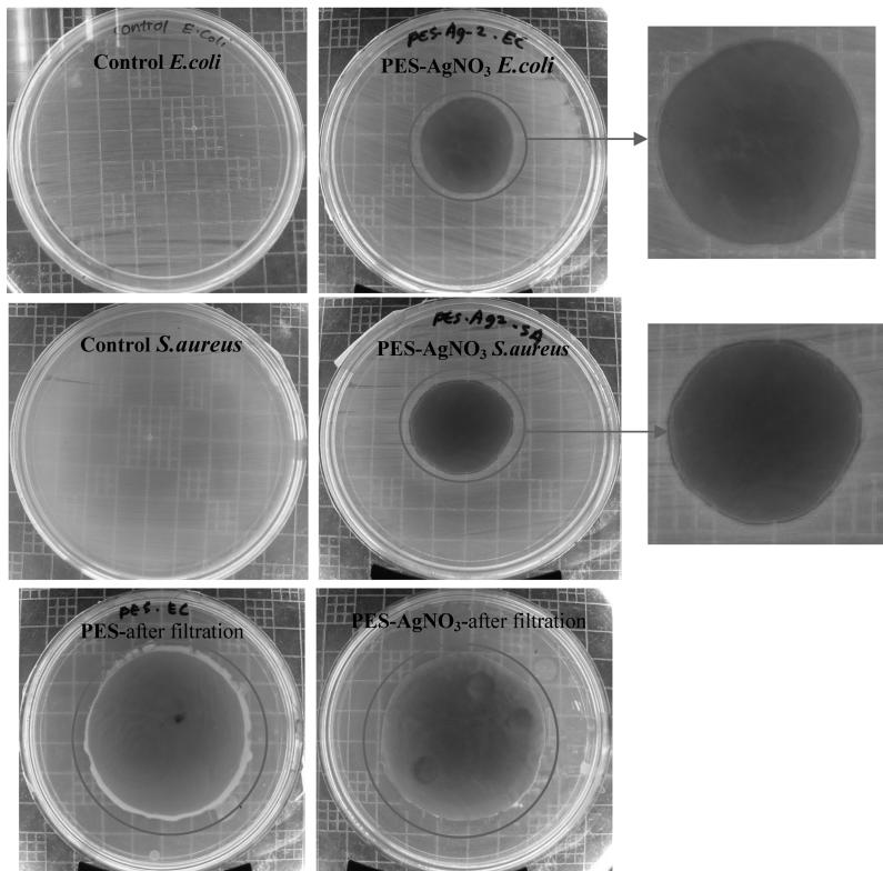
Fig. 8 Photographs of an antibacterial test result of the membranes against *E.coli* and *S.aureus*
