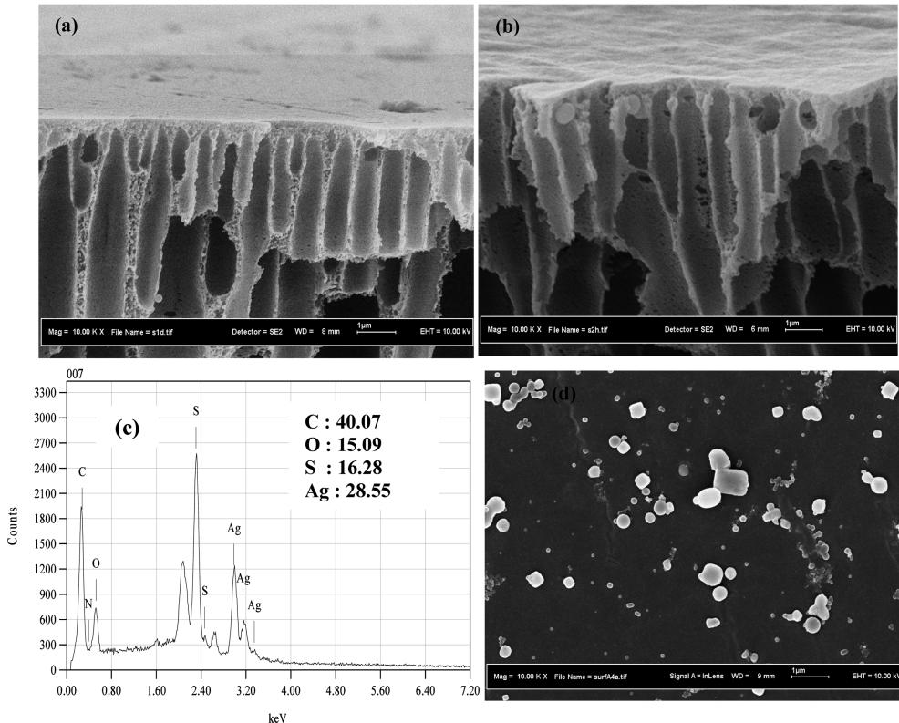
Fig. 5 (a)Cross-section image of PES, (b) Cross-section image of PES -AgNO<sub>3</sub>, (c) Surface image of PES -AgNO<sub>3</sub>, (d) EDX spectra of PES -AgNO<sub>3</sub>(c). The addition of AgNO<sub>3</sub> did not change the morphology of PES membrane as evidenced in the cross sectional image of both membranes (a) and (b)
