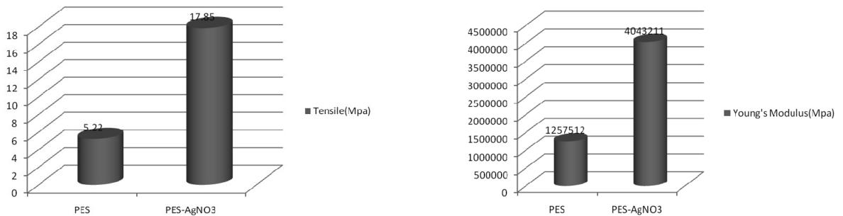
Fig. 7 Mechanical properties of PES and PES-AgNO<sub>3</sub> membranes. Comparison showed mechanical properties of PES membrane improved after loaded with AgNO<sub>3</sub>
