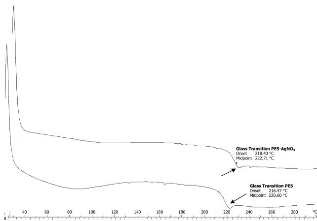
Fig. 4 DSC thermograms of PES and PES- $\text{AgNO}_3$  membranes
