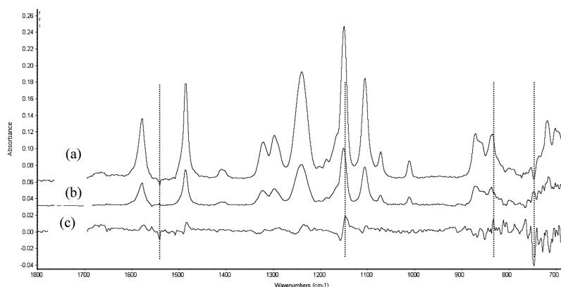
Fig. 1 ATR-FTIR spectra of (a) PES, (b) PES- $\text{AgNO}_3$  and (c) Subtraction of PES- $\text{AgNO}_3$  and PES
