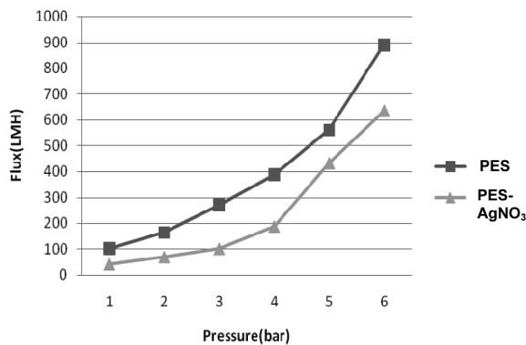
Fig. 6 Pure water permeability ( $\text{Lm}^{-2}\text{hr}^{-1}$ ) for PES and PES-AgNO<sub>3</sub> membranes against pressure (bar)
