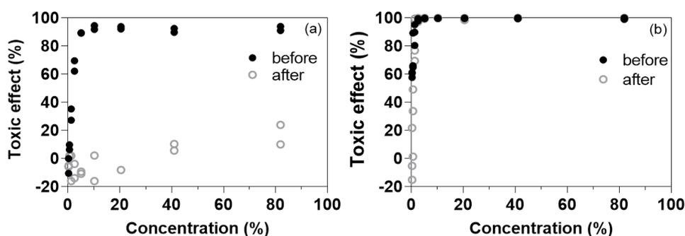
Fig. 4 Changes in the toxic effects on *Aliivibrio fischeri* after 15 min exposure to (a) Pb solution before and after sorption on polyethylene (PE) fragments with additives and (b) Cu solution before and after sorption on PE fragments. The concentrations were expressed as the percentage (v/v) of the initial solution in order to compare the toxicity changes before and after sorption
