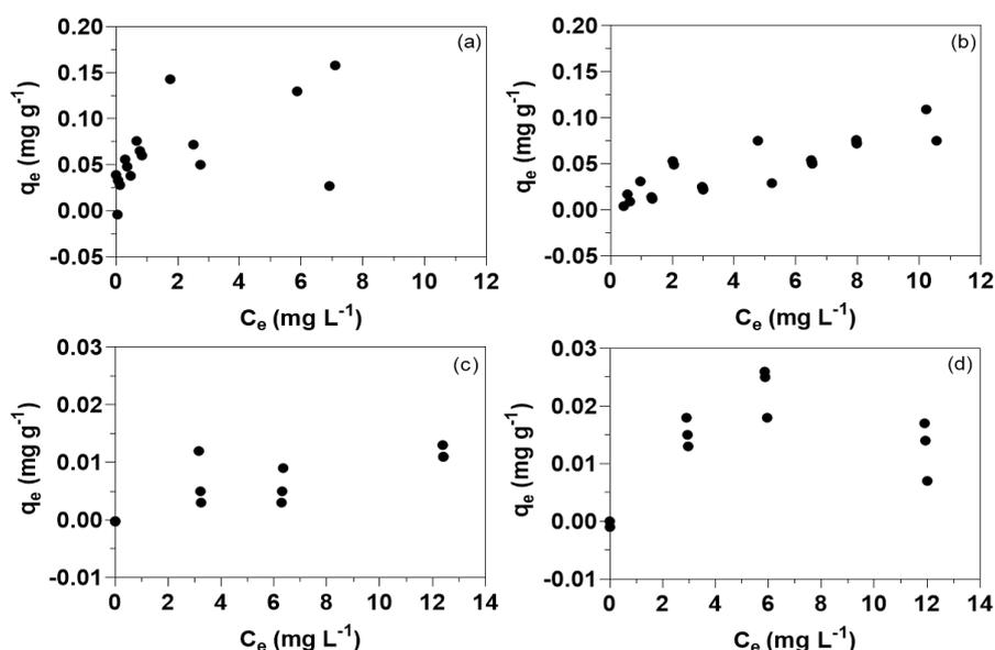
Fig. 3 Data obtained from equilibrium sorption experiments (a) for Pb on polyethylene (PE) fragments with additives, (b) for Pb on PE fragments without additives, (c) for Cu on PE fragments with additives, and (d) for Cu on PE fragments without additives
