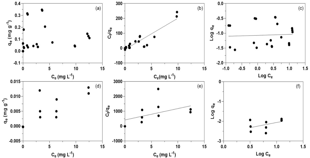
Fig. 2 (a) Data obtained from equilibrium sorption experiments, (b) fitted results to linearized Langmuir isotherm, (c) fitted results to linearized Freundlich isotherm for Cu sorption on polyethylene (PE) films (<5 mm × <5 mm), (d) data obtained from equilibrium sorption experiments, (e) fitted results to linearized Langmuir isotherm, and (f) fitted results to linearized Freundlich isotherm for Cu sorption on PE fragments (<125 μm)
