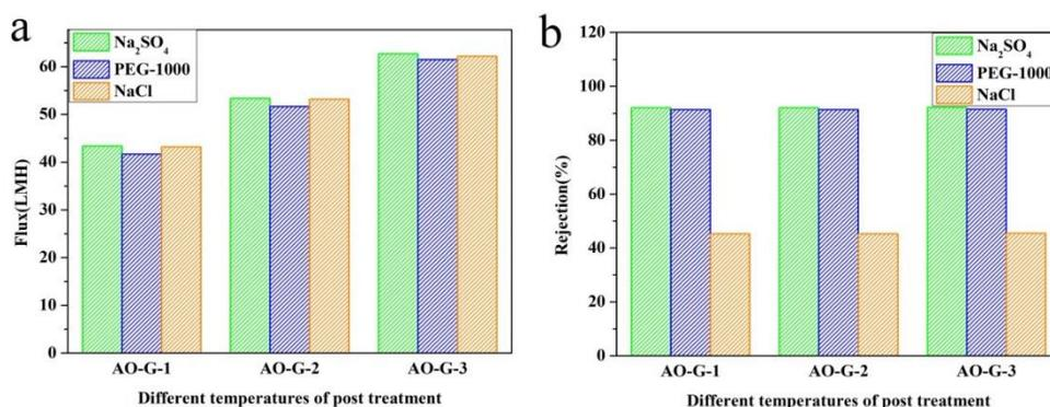
Fig. 9 (a) The flux and (b) Rejection of composite membrane with different temperatures of post treatment
