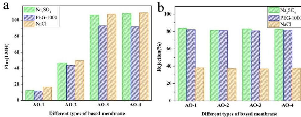
Fig. 2 (a) The flux and (b) Rejection of composite membrane with different types of based membrane
