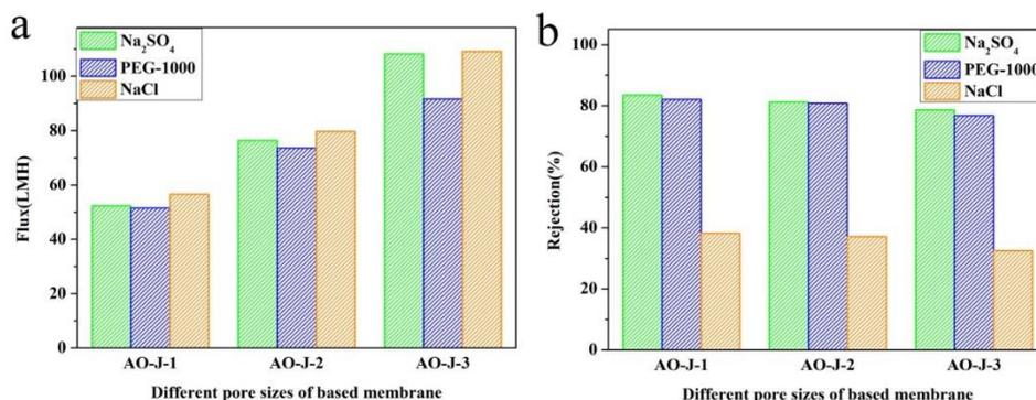
Fig. 4 (a) The flux and (b) Rejection of composite membrane with different pore sizes of based membrane.
