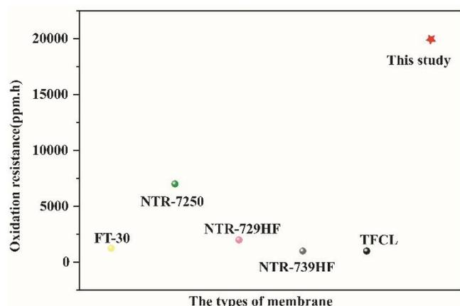
Fig. 12 Performance comparison with other types of membrane
