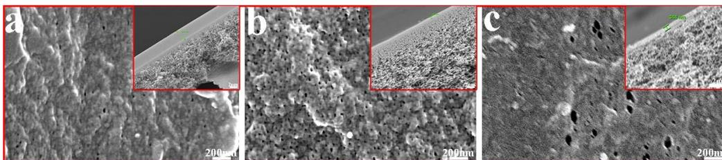
Fig. 3 SEM images of the different pore size of based membrane. (a) 0.04  $\mu\text{m}$ ; (b) 0.06  $\mu\text{m}$ ; (c) 0.08  $\mu\text{m}$ ; The inset images represented the cross-sectional images of the corresponding composite NF membrane, respectively
