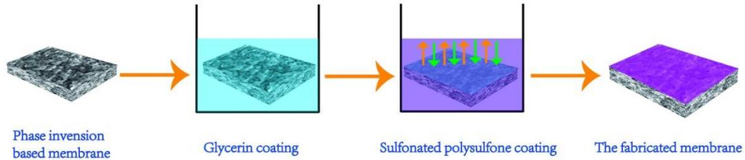
Fig. 1 Schematic diagram for the fabricated NF membrane
