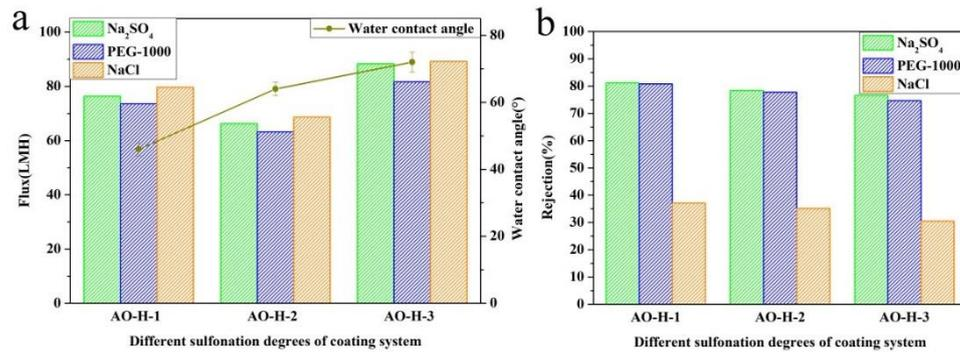
Fig. 5 (a) The flux, water contact angle and (b) Rejection of composite membrane with different sulfonation degrees of coating system
