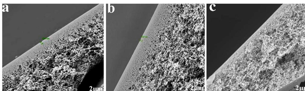
Fig. 10 SEM images of the different temperatures of post treatment progress. (a) nature wind; (b) low temperature air knife; (c) high and low temperature variable frequency air knife
