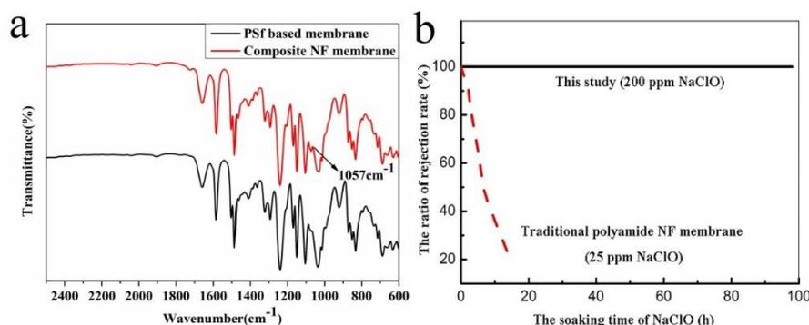
Fig. 11 (a) FTIR and (b) Oxidation resistance of composite NF membranes
