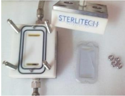
Fig. 6 Cross flow membrane filtration cell (CF042)
