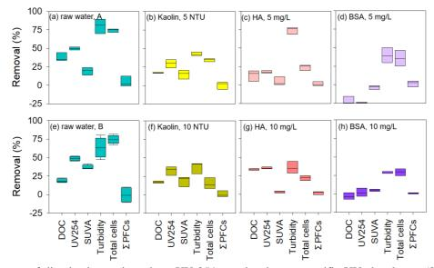
Fig. 1 Removal rates of dissolved organic carbon, UV 254 nm absorbance, specific UV absorbance (SUVA), turbidity, total bacterial cells, and bulk PFCs via coagulation in surface water collected from drinking water treatment plants A and B: raw water (a) and (e), Kaolin (b) and (f), humic acids (HA) (c) and (g), and bovine serum albumin (BSA) (d) and (h)
