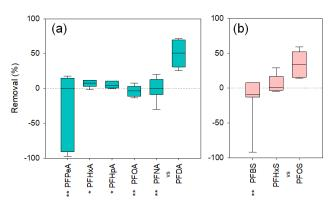
Fig. 2 Perfluorinated compounds removals from the raw waters of drinking water treatment plants A and B via coagulation: (a) perfluorodecanoic acid (PFDA) versus carboxylic species and (b) perfluorooctanesulfonic acid (PFOS) versus sulfonic species. Asterisks represent the significant difference of removal rates (\* and \*\* for p values < 0.05 and < 0.01, respectively).
