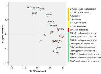
Fig. 4 Principal component analysis in a rotated space. PC1 axis putatively explains the removal mechanisms based on the hydrophobicity and insolubility of pollutants
