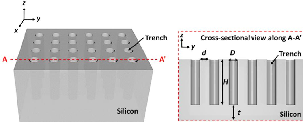
Fig. 1 Schematic illustration of silicon substrate including trenches. Design of silicon structure with the diameter of trench ( $D$ ), the height of trench ( $H$ ), the distance between trenches ( $d$ ), and the thickness of initial bottom layer ( $t$ ).
