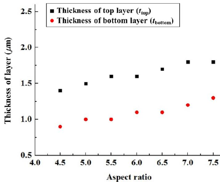
Fig. 3 Thickness of top layer ( $t_{top}$ ) and of bottom layer ( $t_{bottom}$ ) of SON structure with respect to various aspect ratios of the initial trenches.
