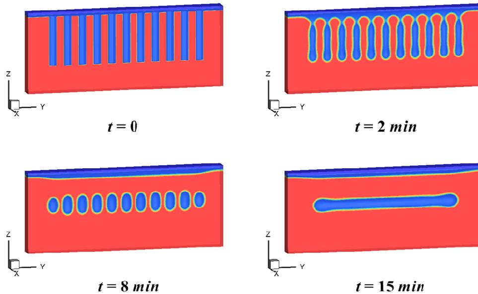
Fig. 2 Time-dependent simulation results for the formation of void-embedded microstructure (i.e., SON structure) during an annealing process. The red and blue regions represent the silicone and air, respectively. Aspect ratio ( $H/D$ ) of the initial trenches is 4.7.
