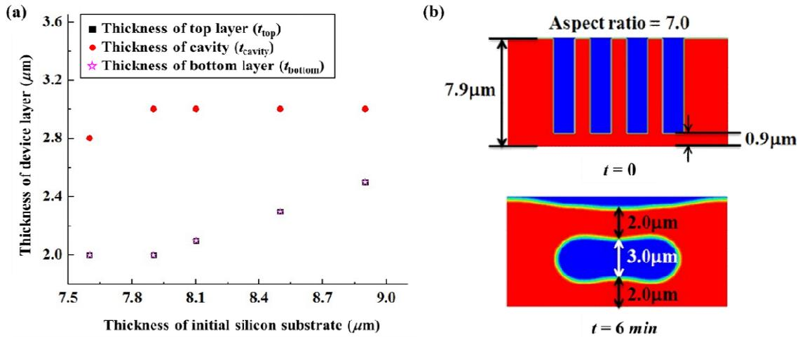
Fig. 5 Different morphological formation of SON structure according to the various design parameters. (a) The position of cavity can be controlled to be located at the center of SON structure (i.e.,  $t_{\text{top}} = t_{\text{bottom}}$ ). (b) The aspect ratio of the initial trench corresponds to the summation of thickness of transformed three layers ( $t_{\text{top}}$ ,  $t_{\text{cavity}}$ , and  $t_{\text{bottom}}$ ).
