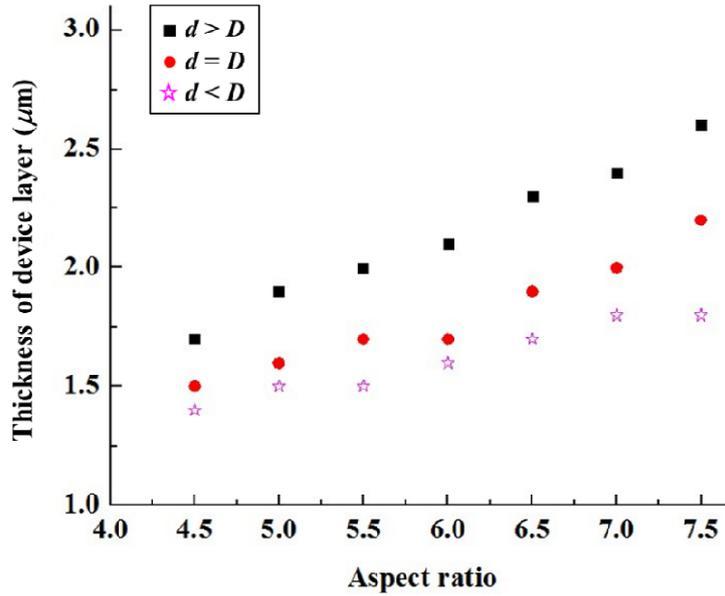
Fig. 4  $t_{\text{top}}$  of SON structure according to the relation between the trench distance ( $d$ ) and the diameter of trench ( $D$ ).  $D$  is fixed as  $1.0 \mu\text{m}$  in all of simulations.
