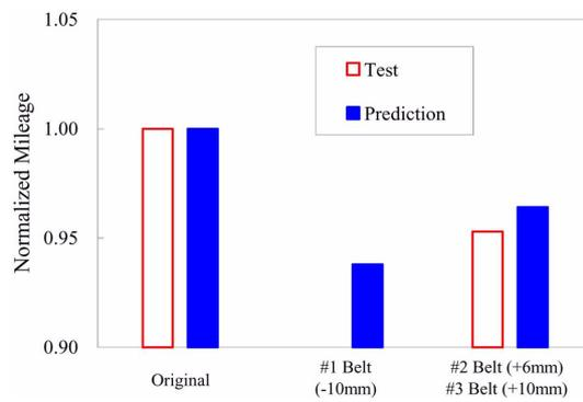
Fig. 10 Comparison of predicted mileage to measurement from tests
