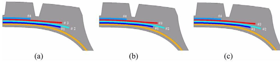
Fig. 8 Design with the different belt width: (a) original belt width, (b) #1 Belt (-10 mm), (c) #2 Belt (+6 mm), #3 belt (+10 mm)
