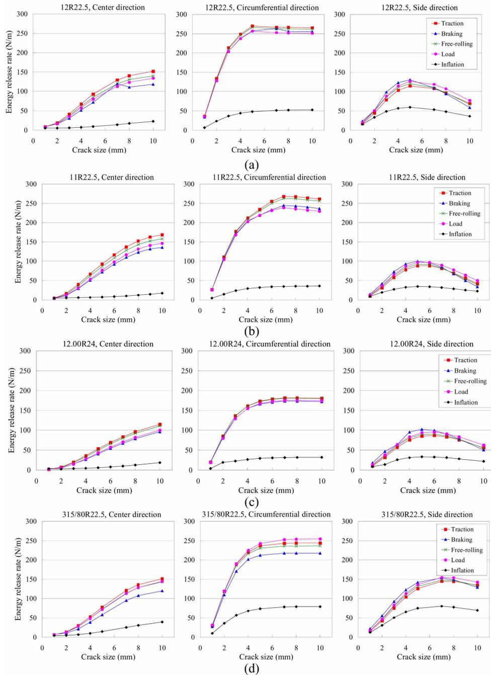
Fig. 7 Energy release rate with respect to the direction of crack propagation for the driving condition: (a) 12R22.5, (b) 11R22.5, (c) 12.00R24, (d) 315/80R22.5 radial truck tires
