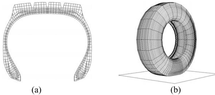
Fig. 2 Global finite element modeling of 12R22.5 tire: (a) 2D model, (b) 3D model
