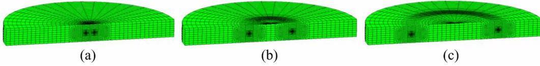
Fig. 4 Local crack model: (a) 1 mm, (b) 5 mm, (c) 10 mm
