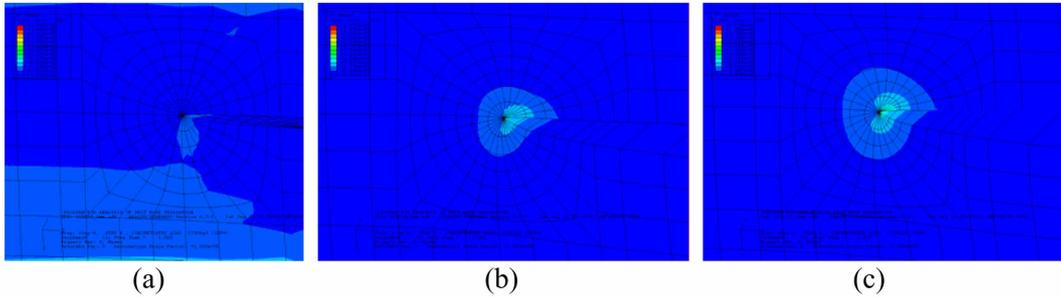
Fig. 5 Stress distribution at the crack tips for a size of 12R22.5: (a) 1 mm, (b) 5 mm, (c) 10 mm
