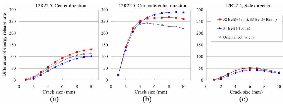
Fig. 9 Difference of energy release rate with respect to the direction of crack propagation: (a) center direction, (b) circumferential direction, (c) side direction
