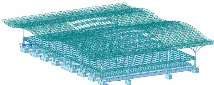
Fig. 2 Station dynamic analysis model
