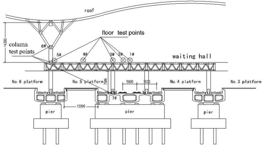
Fig. 8 The layout of station measuring points (1#~7# stand for output points)
