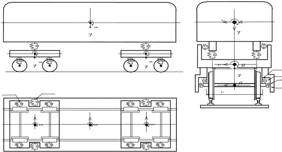
Fig. 3 Vehicle computational model
