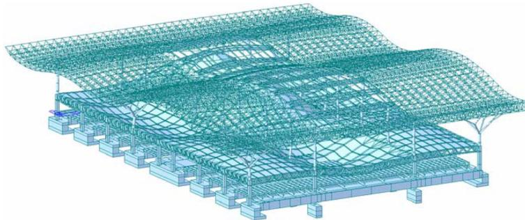
Fig. 7 The 12th mode shape of station (local vibration of waiting hall floor,  $f=2.021$  Hz)
