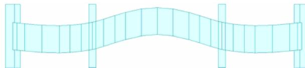
Fig. 5 First lateral mode shape of 30.9 + 49 + 30.9 m continuous beam
