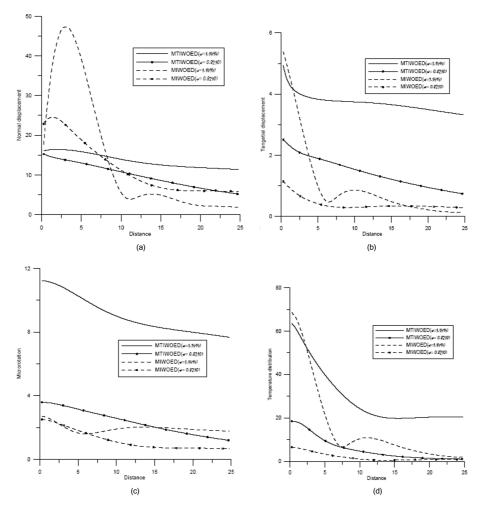
Fig. 4 Variations in the values of (a) normal displacements (b) tangential displacements (c) microrotation (d) temperature distribution of waves with respect to distance
