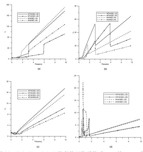
Fig. 1 Variations in the phase velocity (a)  $V_1$  (b)  $V_2$  (c)  $V_3$  (d)  $V_4$  of waves with respect to frequency
