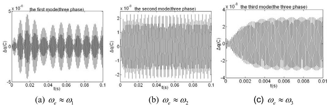
Fig. 6 Forced responses of the electric system to voltage excitation under mechanical disturbance
