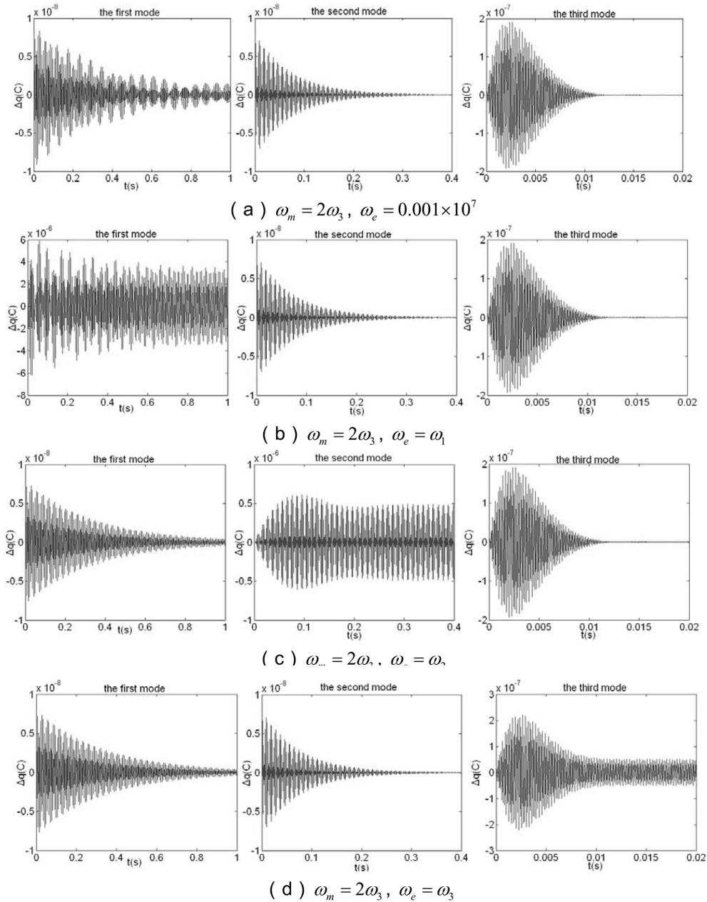
Fig. 9 Coupled vibrations under mechanical disturbance and voltage excitation ( $\omega_m = 2\omega_3$ )
