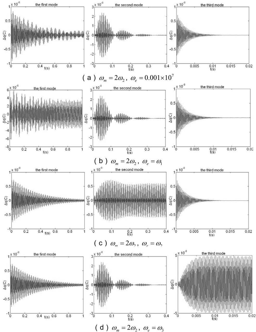
Fig. 8 Coupled vibrations under mechanical disturbance and voltage excitation ( $\omega_m = 2\omega_2$ )
