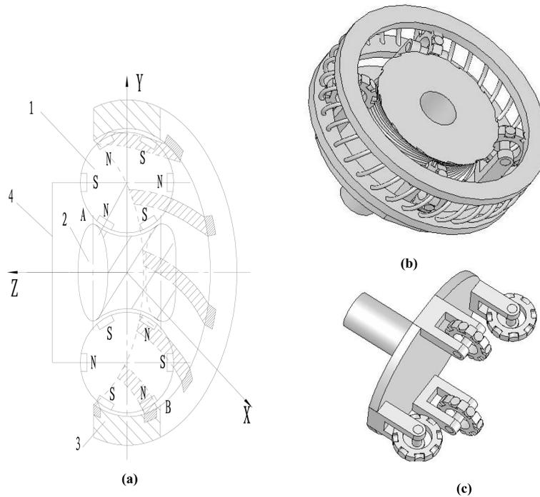
Fig. 1 The electromechanical integrated toroidal drive
