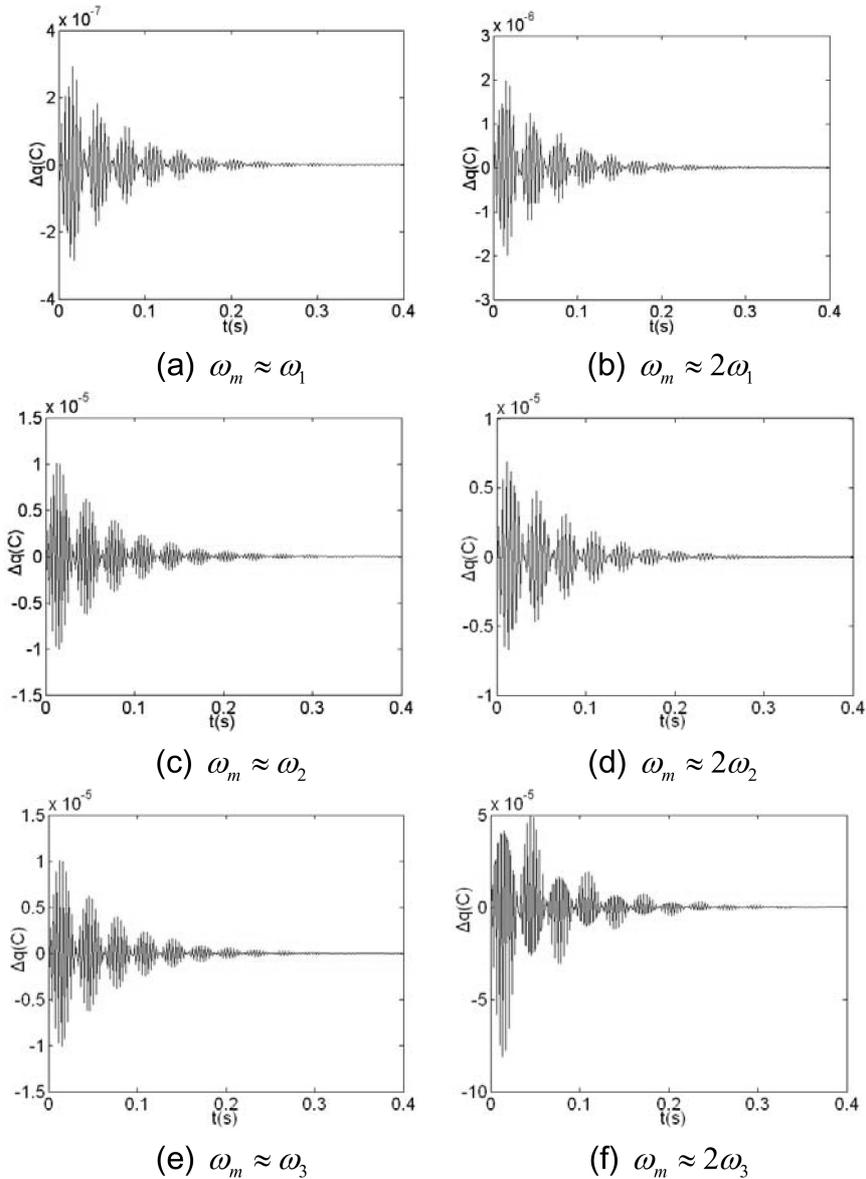
Fig. 5 Resonance vibrations of the electric system under mechanical disturbance
