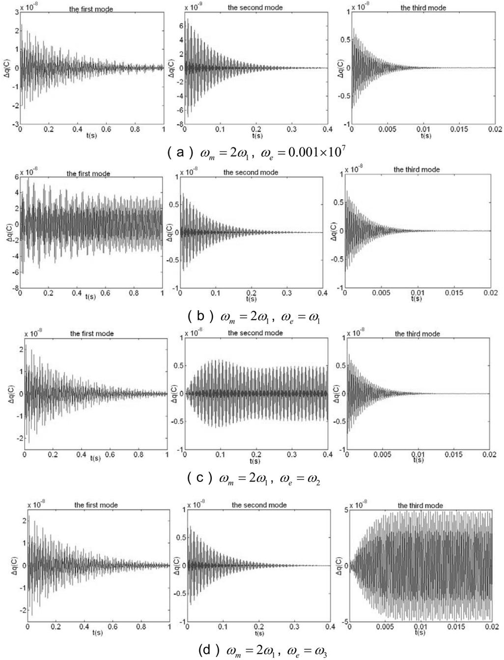
Fig. 7 Coupled vibrations under mechanical disturbance and voltage excitation ( $\omega_m = 2\omega_1$ )
