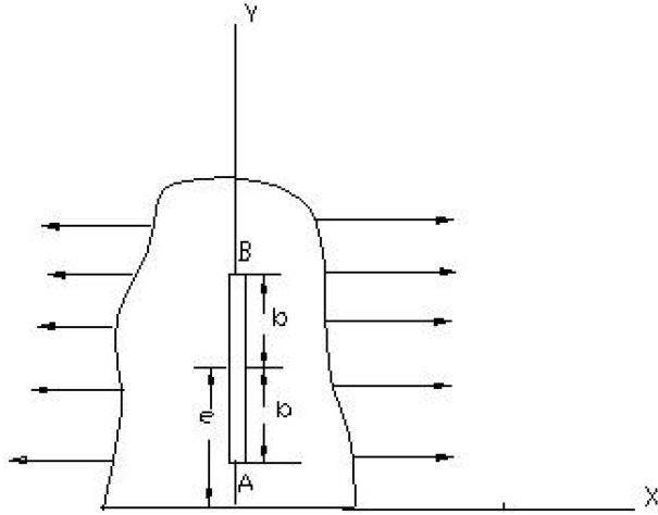
Fig. 1 Crack in semi-infinite plate
