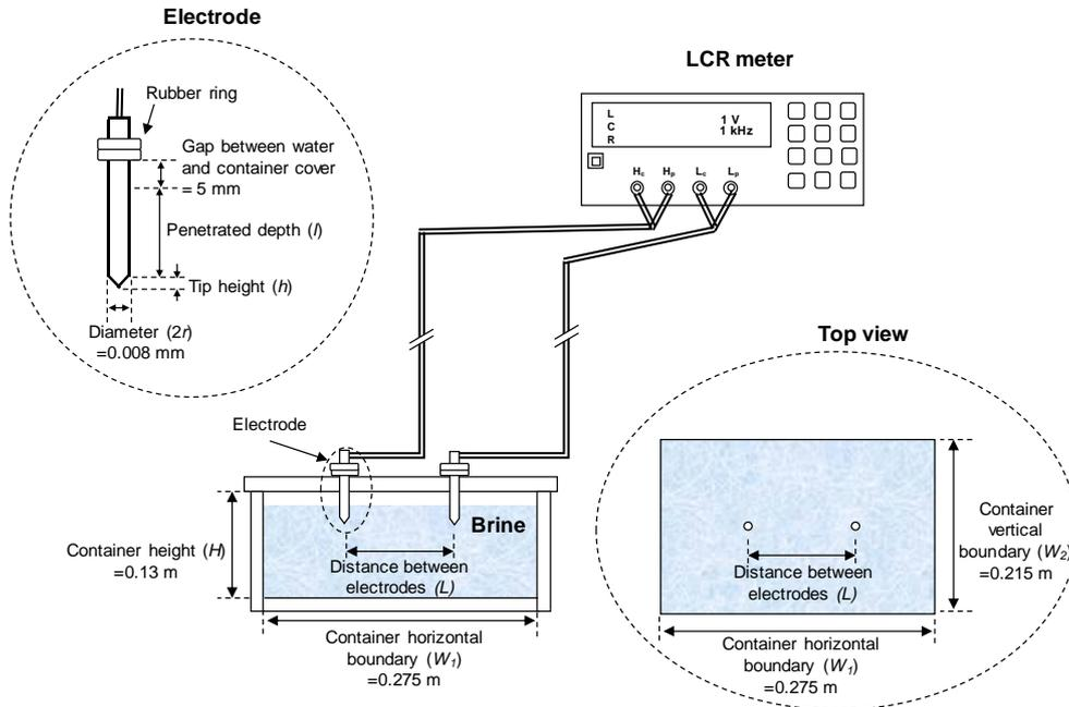
Fig. 4 Test setup: measurement equipment, container and electrodes
