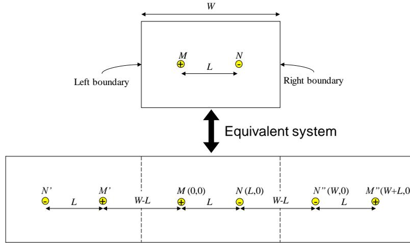
Fig. 3 Equivalent system with imaginary electrodes (Hong *et al.* 2019)
