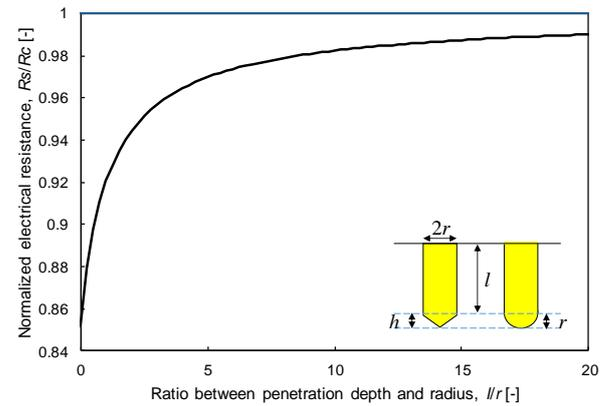
Fig. 6 Effect of penetration depth on the electrical resistance of spherical and conical tip cylindrical electrodes. Distance between two electrodes is fixed as 0.085 m
