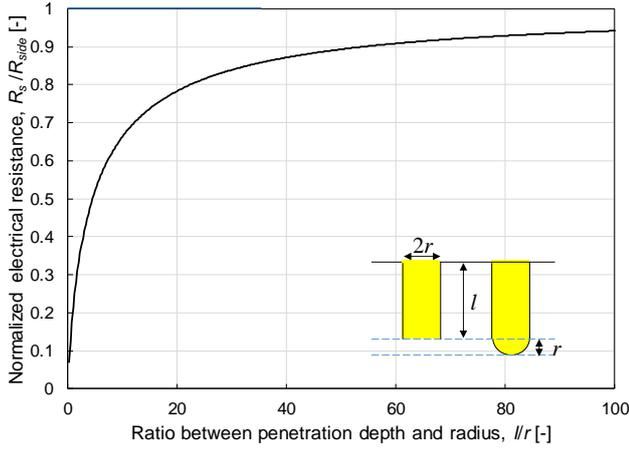
Fig. 7 Effect of tip on the measured electrical resistance. Distacne between two electrodes is fixed as 0.085 m
