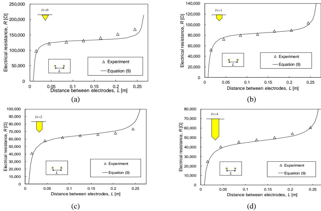
Fig. 5 Electrical resistance of different distance and depth: (a)  $l/r=0$ , (b)  $l/r=1$ , (c)  $l/r=2$ , and (d)  $l/r=4$ . Radius ( $r$ ) and tip height ( $h$ ) are fixed as 0.004 m. and penetration depth ( $l$ ) varies from 0 to 0.016 m
