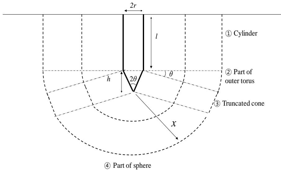
Fig. A1 Symbols of the cylindrical electrodes with conical tip
