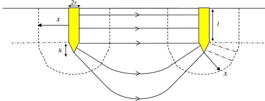
Fig. 2 Definitions of the symbols and equipotential surface shape between two cylindrical electrodes with conical tip
