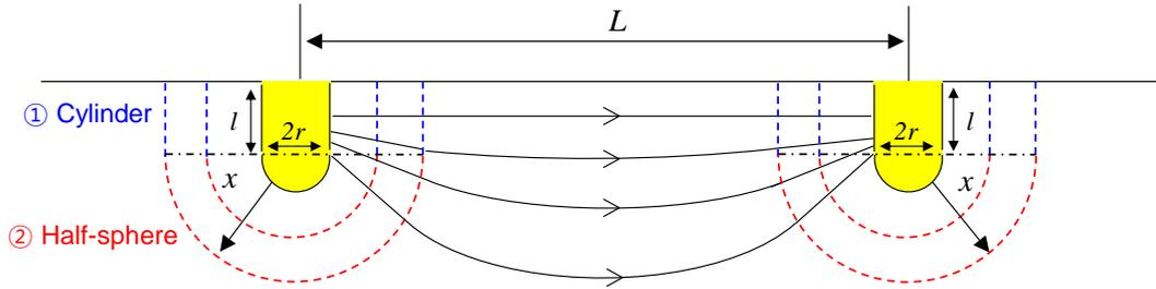
Fig. 1 Definitions of the terms and shape of equipotential surface between two cylindrical electrodes with spherical tip (Modified from Hong *et al.* 2019)
