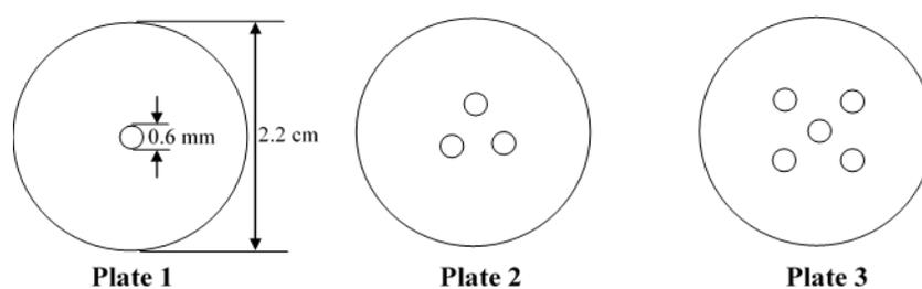
Fig. 2 Orifice plates with different numbers of holes
