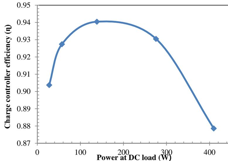
Fig. 5 Power at DC load vs Charge controller efficiency
