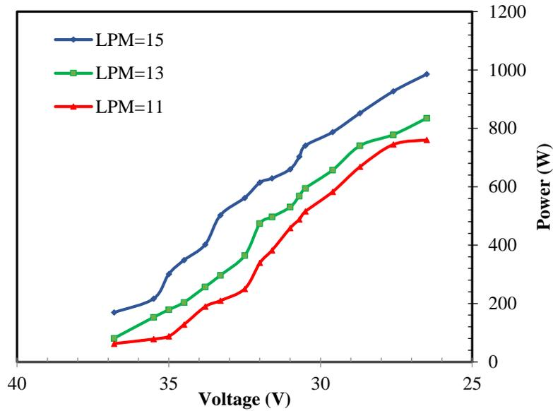
Fig. 4 Characteristics of fuel cell at different flow rate of hydrogen
