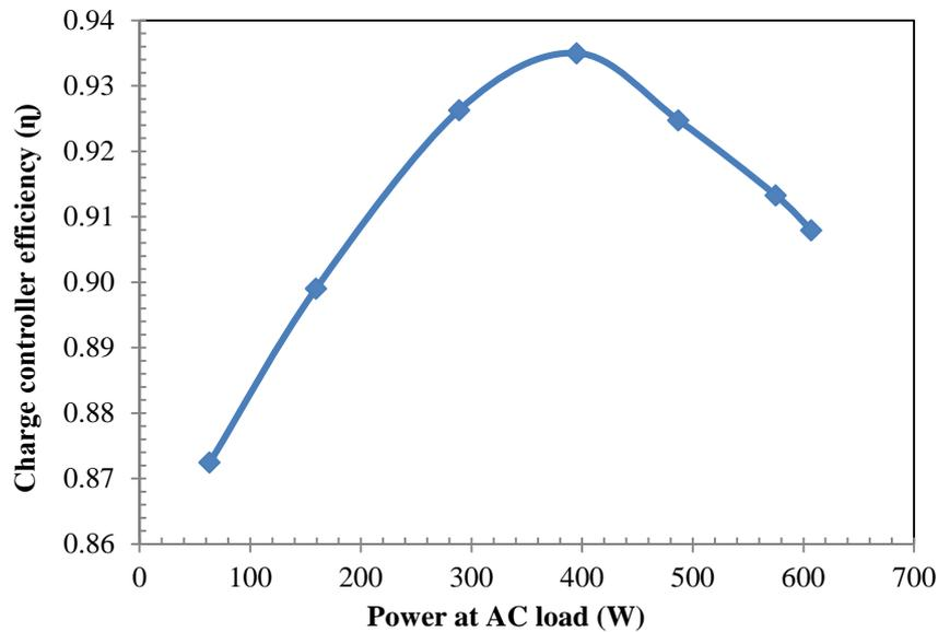
Fig. 6 Power at AC load vs Charge controller efficiency
