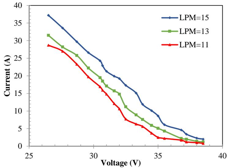
Fig. 3 V-I characteristics of fuel cell
