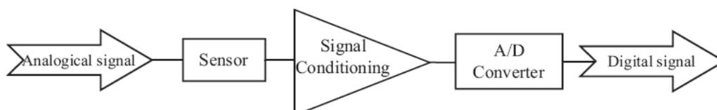
Fig. 1 The basic block diagram of a simple DAQ system
