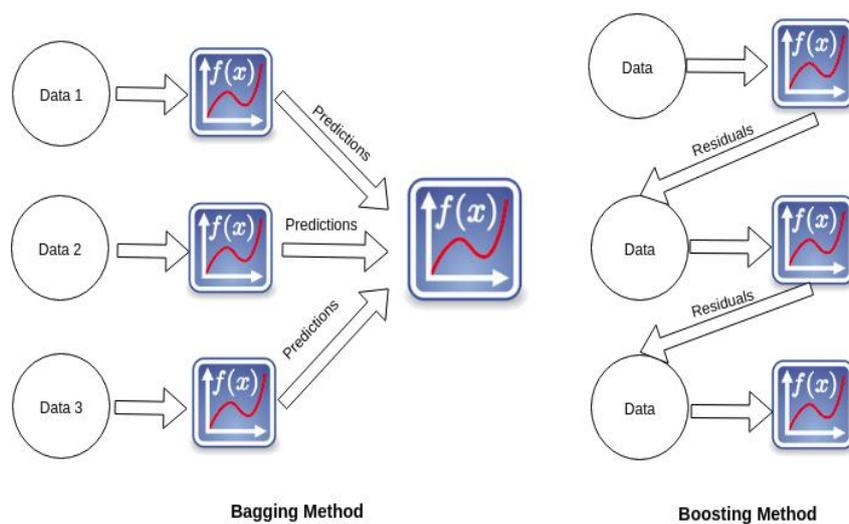
Fig. 1 Difference between bagging and boosting methods
