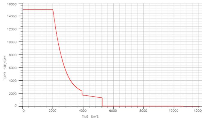
Fig. 7 Reservoir oil production rate
