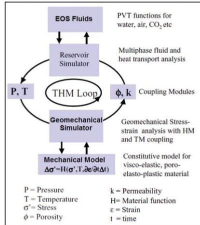
Fig. 3 THM loop (linking between ECLIPSE and ABAQUS)
