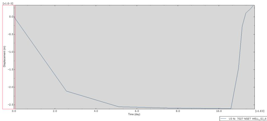
Fig. 14 Vertical displacement around WELL6
