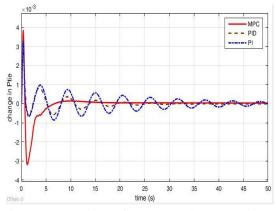
Fig. 15 Change in  $P_{tie}$  for -3% step increment in  $P_{L2}$
