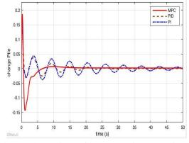
Fig. 12 Change in  $P_{tie}$  for -3% step increment in  $P_{L1}$
