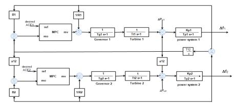
Fig. 3 Proposed two-area LFC scheme by using MPC
