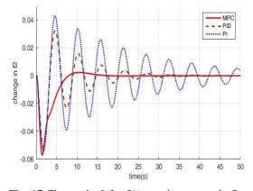
Fig. 16 Change in  $f_1$  for 5% step increment in  $P_{L1}$
