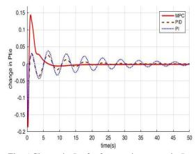
Fig. 6 Change in  $P_{tie}$  for 3% step increment in  $P_{L1}$
