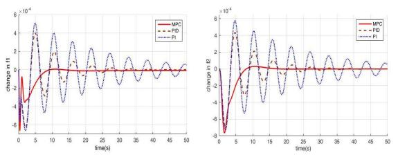
Fig. 7 Change in  $f_1$  for 3% step increment in  $P_{L2}$
