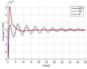
Fig. 9 Change in  $P_{tie}$  for 3% step increment in  $P_{L2}$
