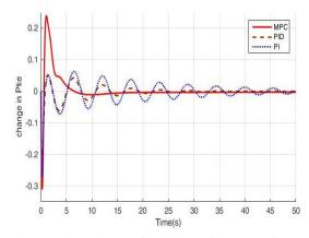
Fig. 18 Change in  $P_{tie}$  for 5% step increment in  $P_{L1}$
